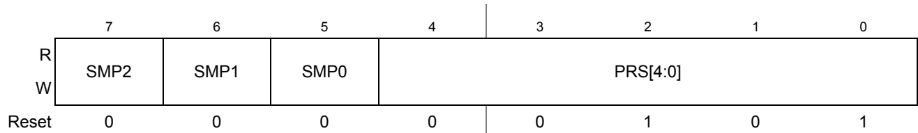
Figure 16-7. ATD Control Register 4 (ATDCTL4)
