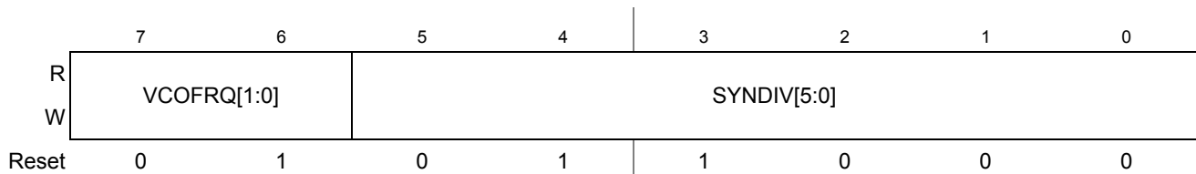
Figure 10-4. S12CPMU Synthesizer Register (CPMUSYNR)
