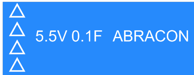
Example of the Markings of a 5.5V 0.1F capacitor
