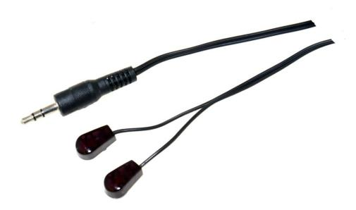
The single jack plug drives two IR emitter wands. The emitters are extremely tiny and are supplied with double sided adhesive pads to affix directly to the equipment fascia. The emitters actually flash red as the IR signal is emitted giving visual confirmation that the IR signal was received and transmitted correctly.
