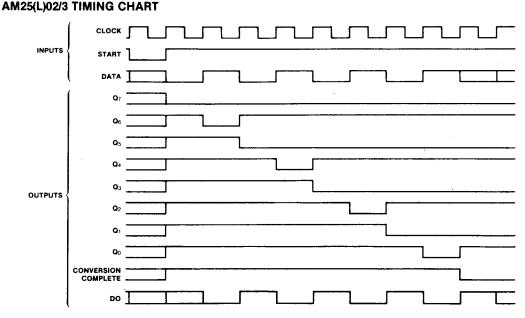
Note: Arbitrary Conversion shown. Timing chart for AM25(L)04 is extended to include 12 outputs, starting with Q<sub>11</sub>.
