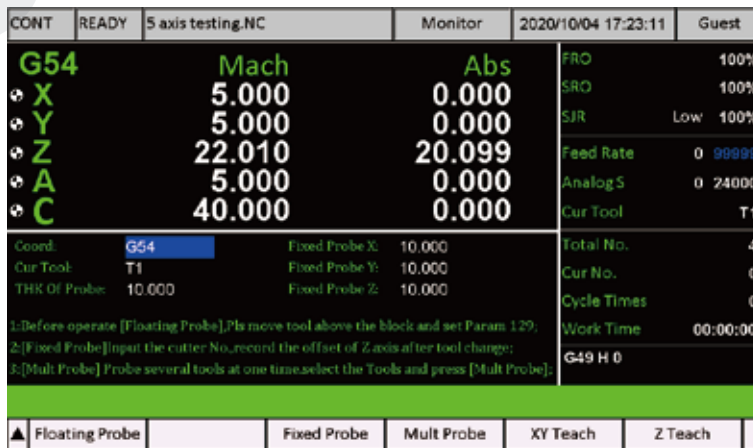
Figure 5-42 Floating Probe Finished
