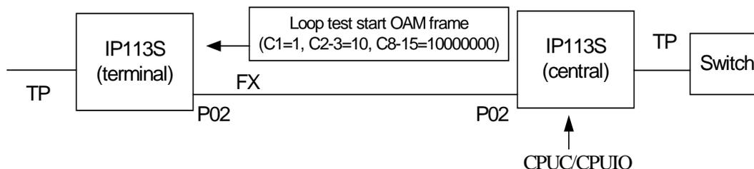
2. Terminal IP113S runs at loop back mode and acknowledges with maintenance frame
