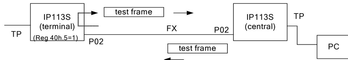
4. PC reports the loop back test result after sending all test frames.
