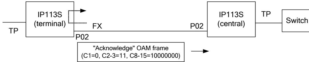
3. Central IP113S forces test frames to terminal IP113S and terminal IP113S loops back the test frames. Central IP113S checks the received test frame.
