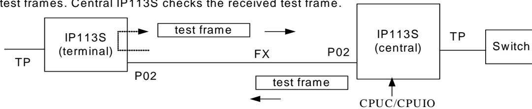
4. Central IP113S ends loop back test enables receive function of TP port and enable T2 timer of terminal IP113S.
