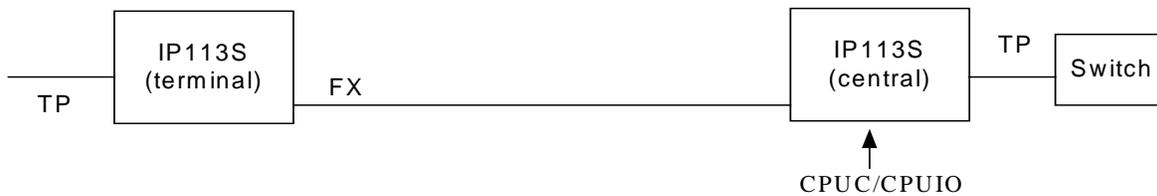
**Start an auto in-band loop back test without programming (by pin)**
