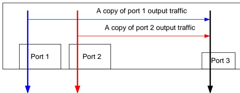
If user wants to monitor the input traffic of port 1 and port 2 from port 3 as shown in the following figure. He has to write “100” to register 19h[8:6] to choose port 3 as a monitoring port and write “001010” to register 19h[5:0] to make the input traffic of port 1 and 2 to be monitored. IP113S LF copy the input traffic of port 1 and port 2 to port 3.
