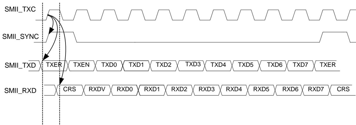
It is note that both SMII\_SYNC and SMII\_TXC are input signals and are shared with all IP113S LF as shown in the following figure.
