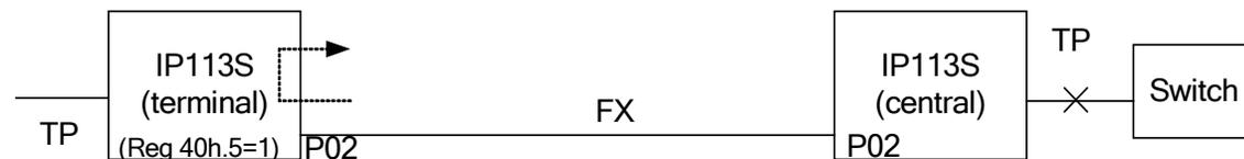
3. PC forces test frames to central IP113S and terminal IP113S loops back the frames.
