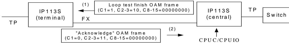
5. To get test result by reading register 40h[7]. All user has to do is step 1 and step 5. From step 2 to step 4 are performed by IP113S automatically.
