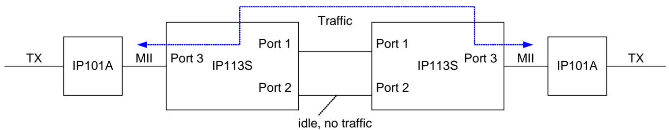
If the fibers on port 1 is broken, traffic is switched from port 1 to port 2 automatically less than 1ms
