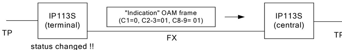
Terminal IP113S LF supports option B, which can inform speed, duplex, and auto-negotiation in terminal IP113S LF. In another words, the information of speed, duplex and auto-negotiation will be replaced by masked data, if terminal IP113S LF is operating in non-option B.
