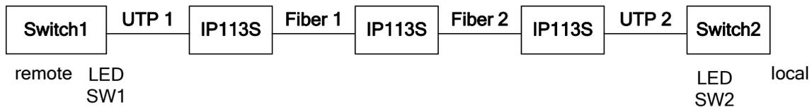
LED SW1 and LED SW2 are both off, if either UTP1, Fiber1, Fiber2 or UTP2 is broken and link fault pass through is enabled. That is, if link status is ok on switch port then all segments are guaranteed link good.
