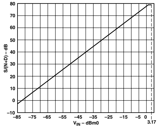
Figure 5d. S/(N+D) vs. V_{IN} (DAC @ 5 V) over Voiceband Bandwidth (300 Hz – 3.4 kHz)
