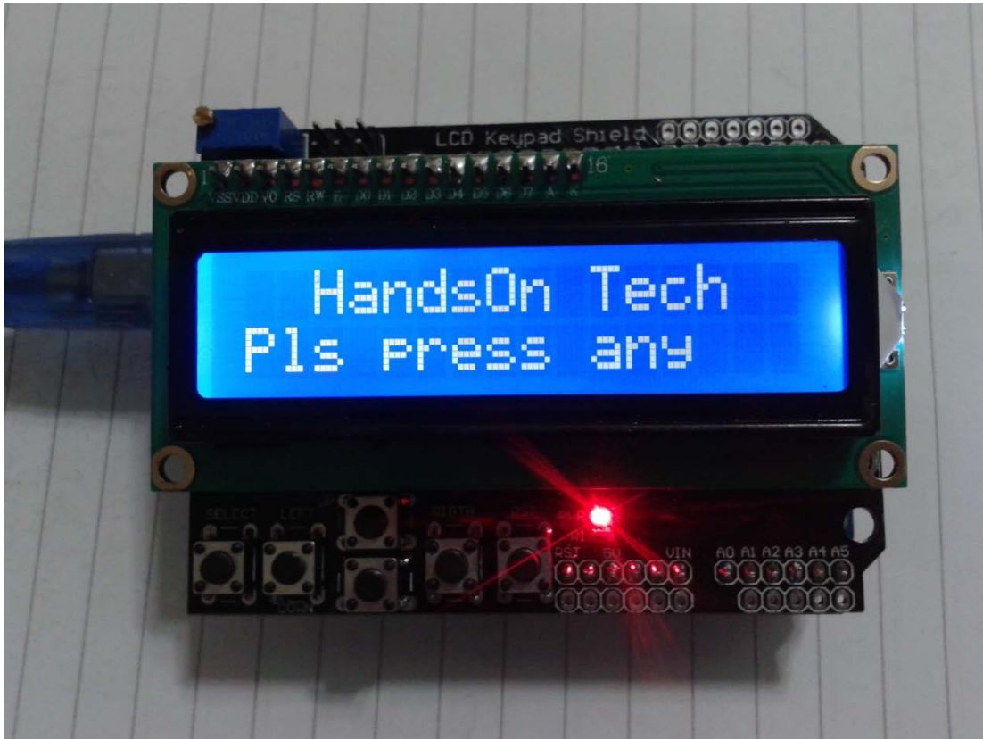
Fig 4.1: Display with code Listing4.1: LCD+Keypad Sketch running.
