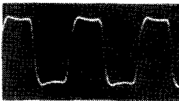
Fig. 17(b) - CA3070 terminal No. 7, oscillator waveform 1.4 V p-p 3.58 MHz.
