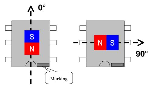
Marking side defines the N polar as 0  $^\circ$  , the Output Voltage (AOUT) decreases as the magnet rotates clockwise.
