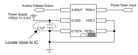
\*Bypass capacitor must be inserted between VDD and VSS.
