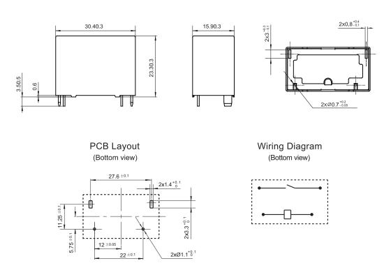
Remark: 1) In case of no tolerance shown in outline dimension: outline dimension ≤1mm, tolerance should be ±0.2mm; outline dimension >1mm and ≤5mm, tolerance should be ±0.3mm; outline dimension >5mm, tolerance should be ±0.4mm.
