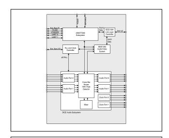
**DICE JR** is a monolithic CMOS ASIC capable of receiving and transmitting up to 64 channels of audio data in accordance with the **IEEE 1394** standard. DICE JR also functions as a cross bridge switch between any combination of **AES3**, **ADAT®**, ADC and DAC ports. The DICE JR technology simplifies the interface to IEEE 1394 and other popular digital audio formats, while it maximizes the clocking accuracy of audio samples.
