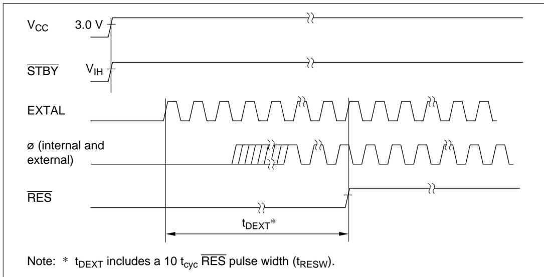
Figure 6.13 External Clock Output Stabilization Delay Time
