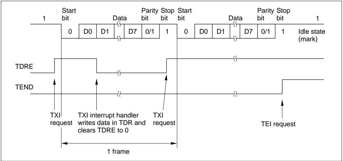
**Figure 12.6 Example of SCI Transmit Operation
