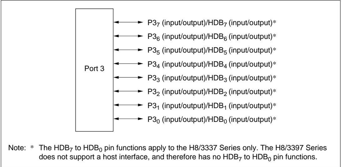
**Figure 7.11 Pin Functions in Mode 3 (Port 3)**
