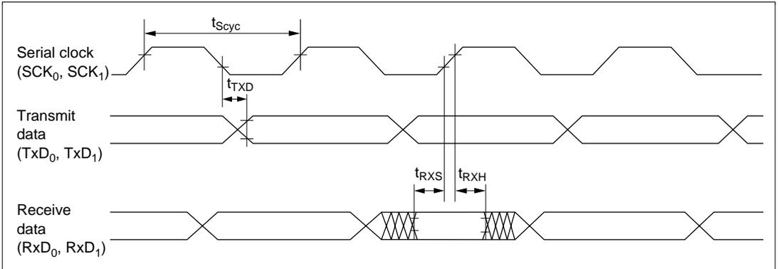
Figure 23.19 SCI Input/Output Timing (Synchronous Mode)
