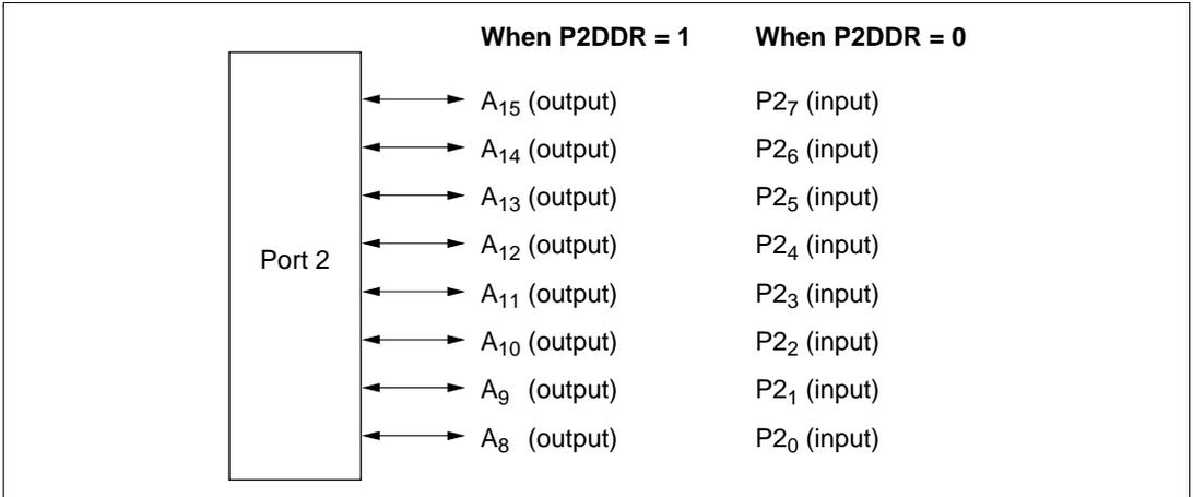
**Figure 7.7 Pin Functions in Mode 2 (Port 2)**
