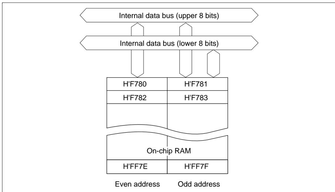
**Figure 17.1 Block Diagram of On-Chip RAM (H8/3337Y)**
