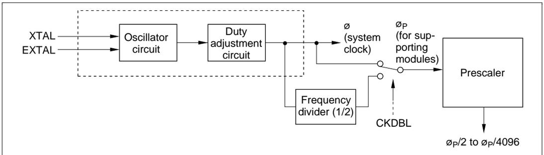
**Figure 6.1 Block Diagram of Clock Pulse Generator**
