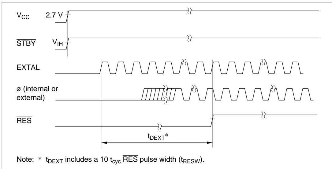
Figure 6.7 External Clock Output Settling Delay Time
