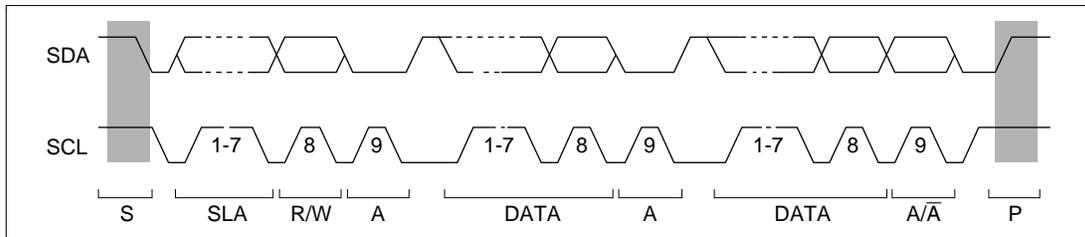
**Figure 13.5 I<sup>2</sup>C Bus Timing**
