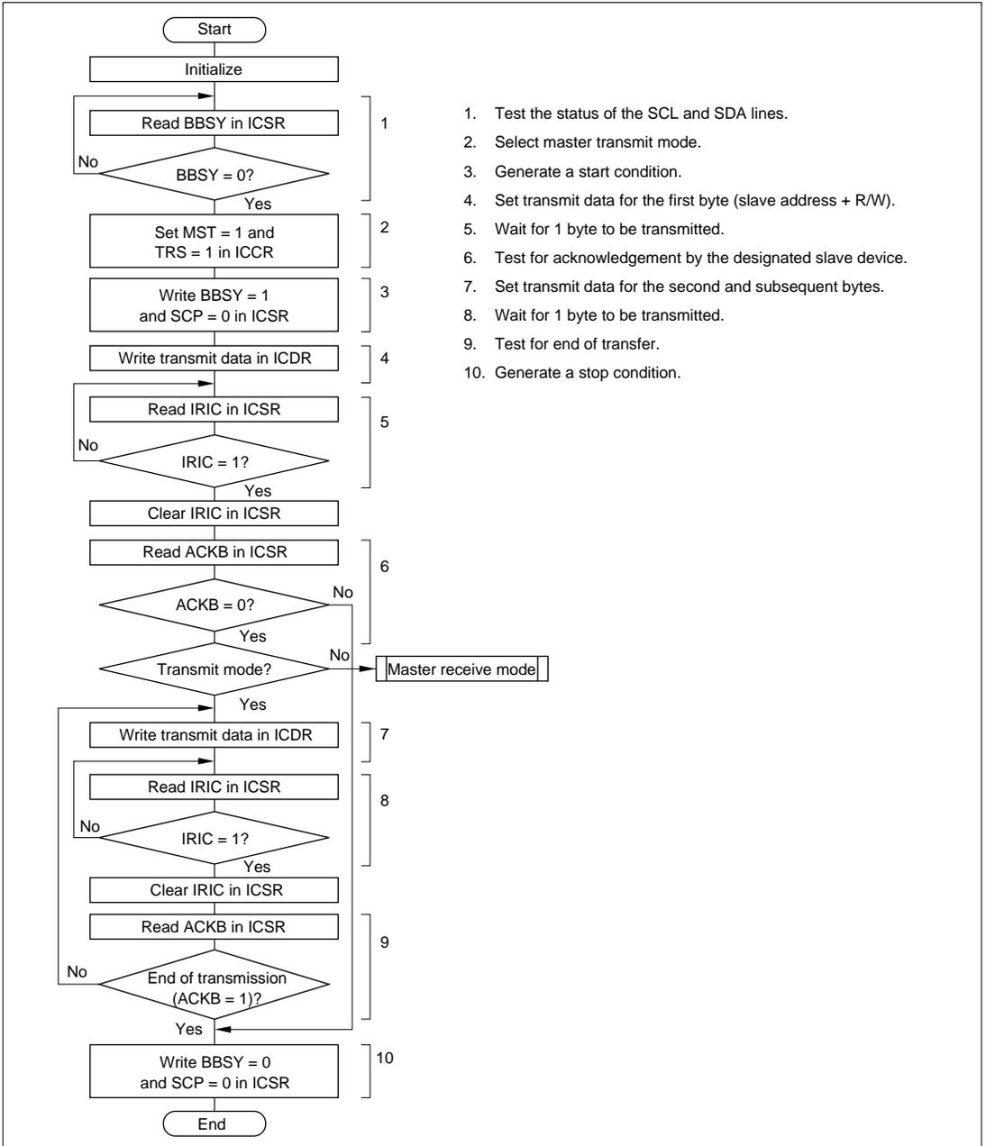
**Figure 13.12 Flowchart for Master Transmit Mode (Example)**
