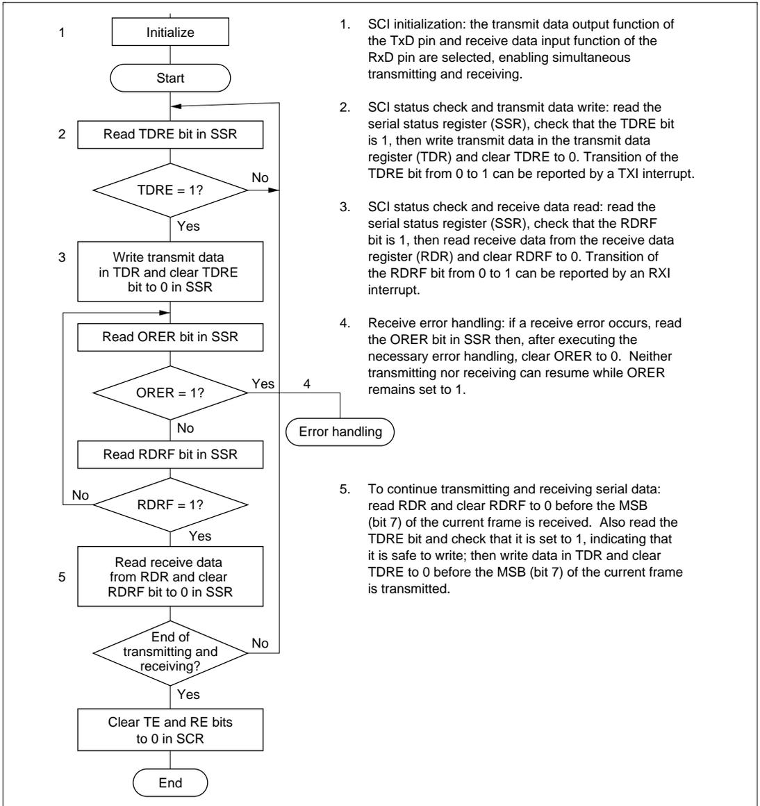
**Figure 12.17 Sample Flowchart for Serial Transmitting and Receiving**
