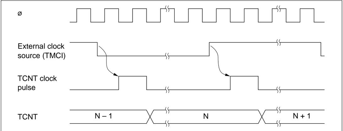
**Figure 9.3 Increment Timing for External Clock Input**
