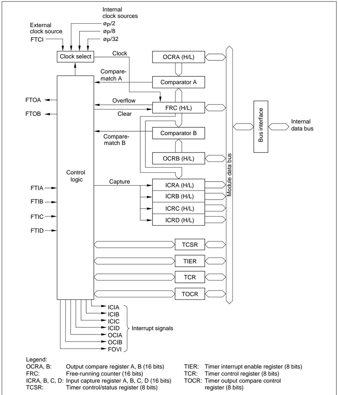
**Figure 8.1 Block Diagram of 16-Bit Free-Running Timer**
