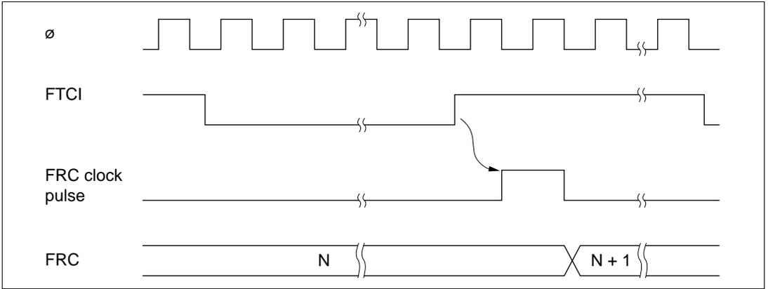
**Figure 8.5 Increment Timing for External Clock Source**
