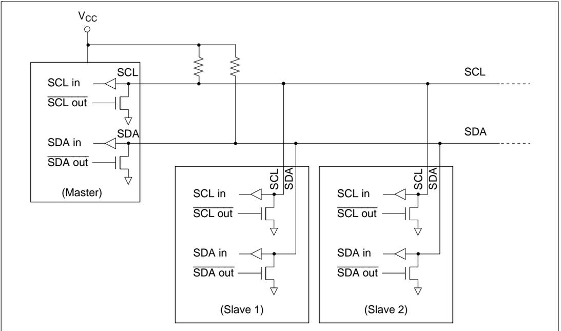
**Figure 13.1 I<sup>2</sup>C Bus Interface Connections (Example) (H8/3337 Series Chip as Master)**
