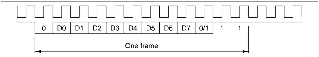
**Figure 12.3 Phase Relationship between Clock Output and Transmit Data
