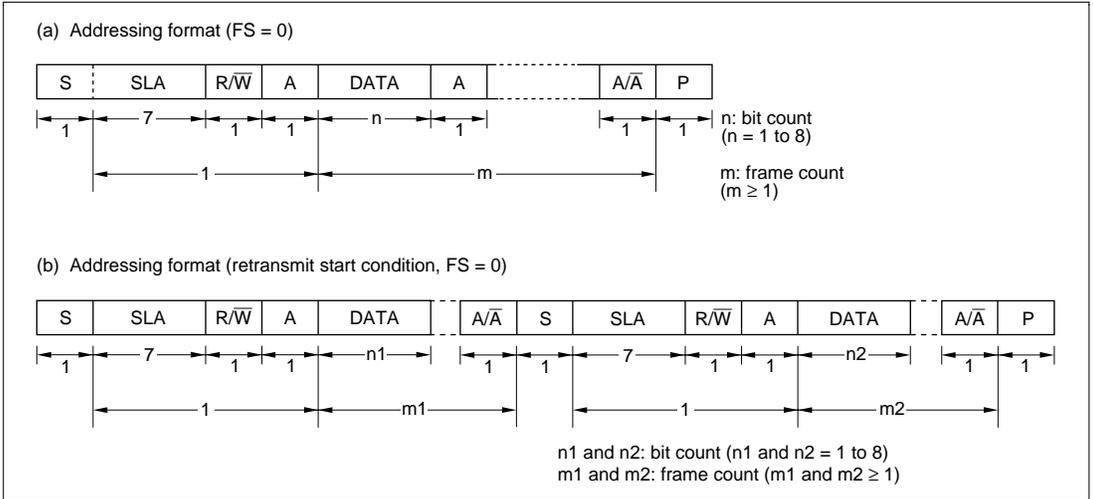
**Figure 13.3 I<sup>2</sup>C Bus Data Formats (Acknowledge Formats)**
