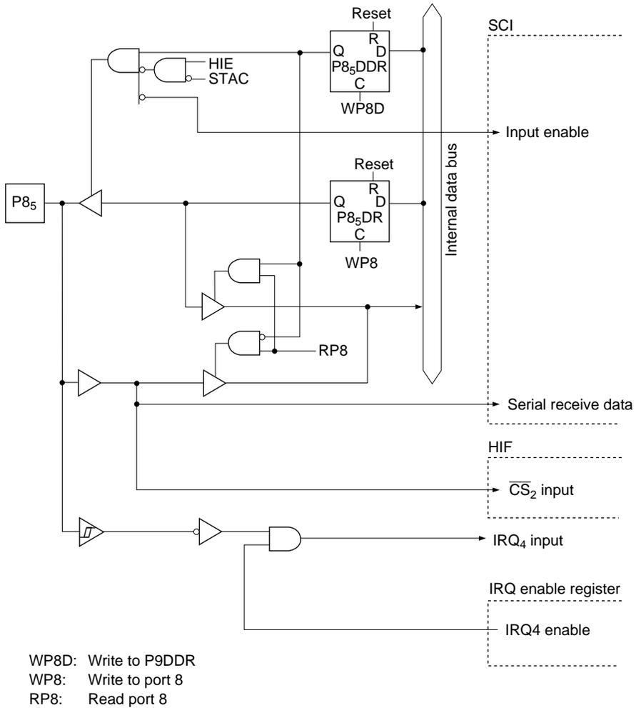
**Figure C.8 (e) Port 8 Block Diagram (Pin P8<sub>5</sub>)**
