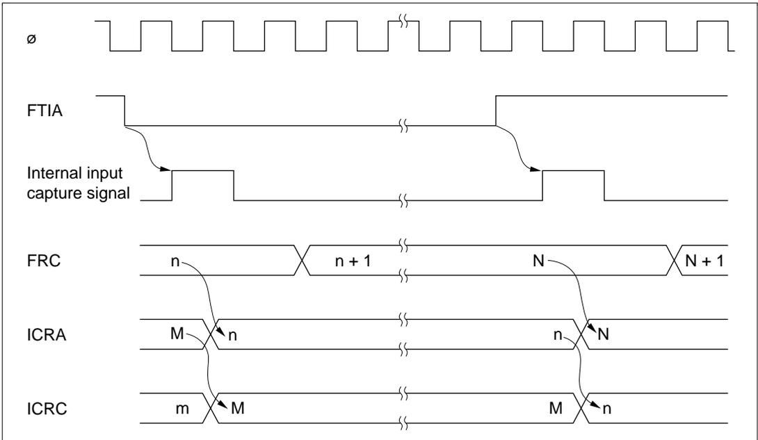
**Figure 8.10 Buffered Input Capture with Both Edges Selected**
