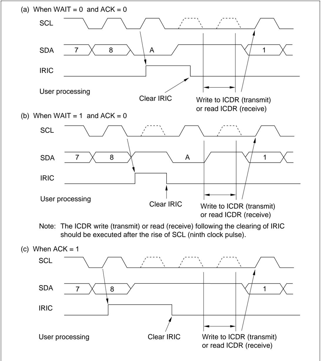
Figure 13.10 IRIC Set Timing and SCL Control
