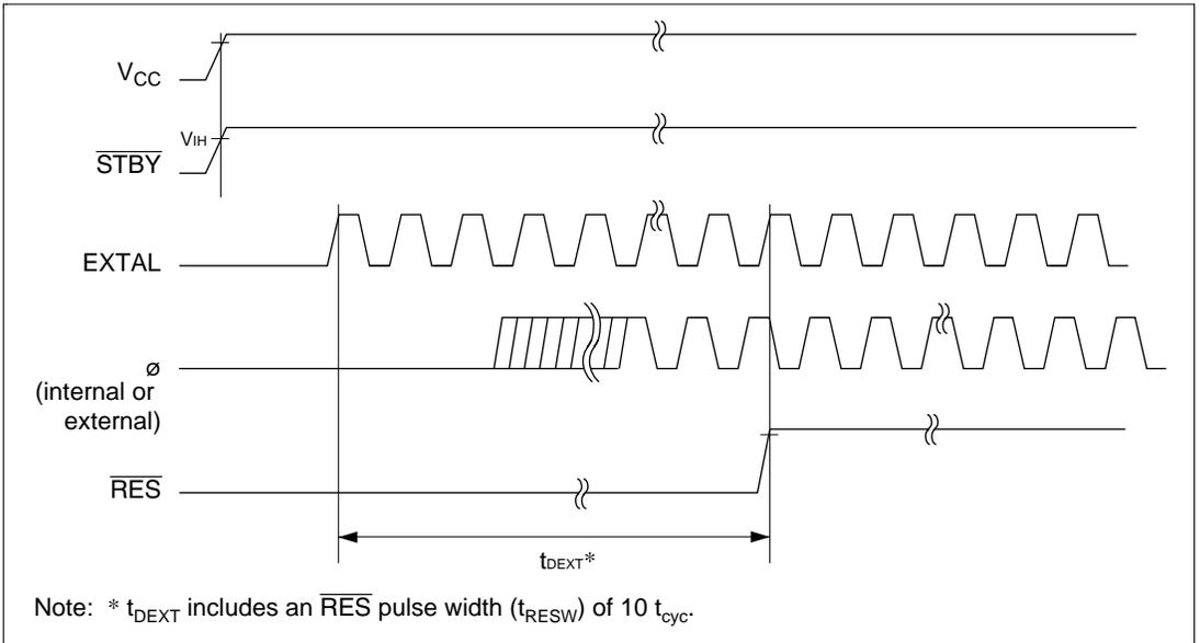
**Figure 23.25 External clock output delay Timing**
