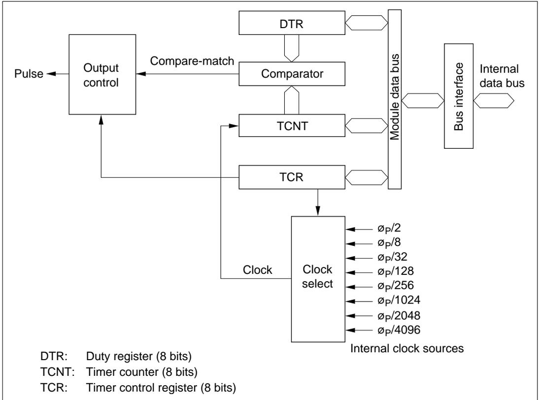
**Figure 10.1 Block Diagram of PWM Timer (One Channel)**
