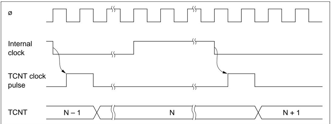
**Figure 9.2 Increment Timing for Internal Clock Input**
