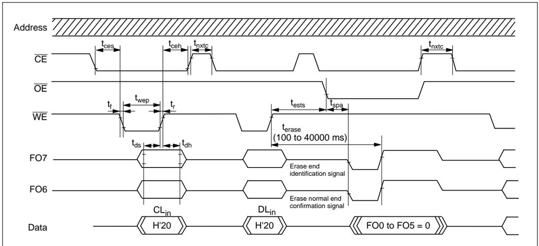
**Figure 21.21 Auto-Erase Mode Timing Waveforms**
