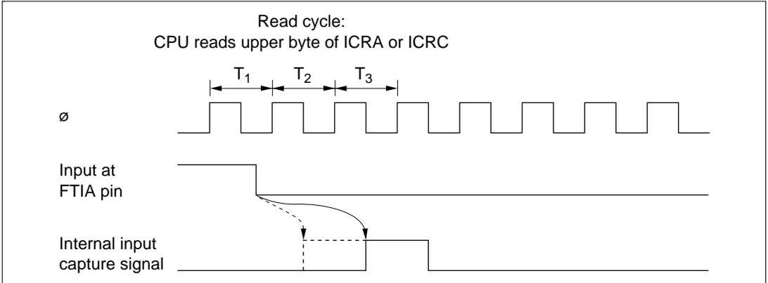
**Figure 8.11 Input Capture Timing (1-State Delay, Buffer Mode)**
