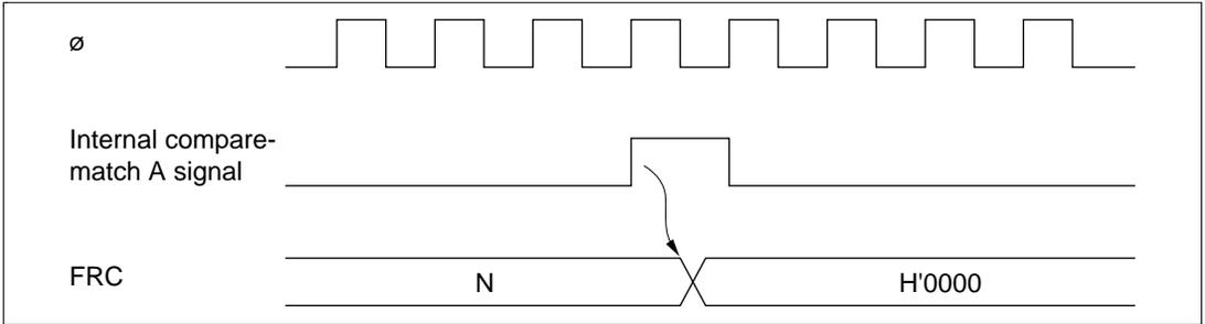
**Figure 8.7 Clearing of FRC by Compare-Match A**
