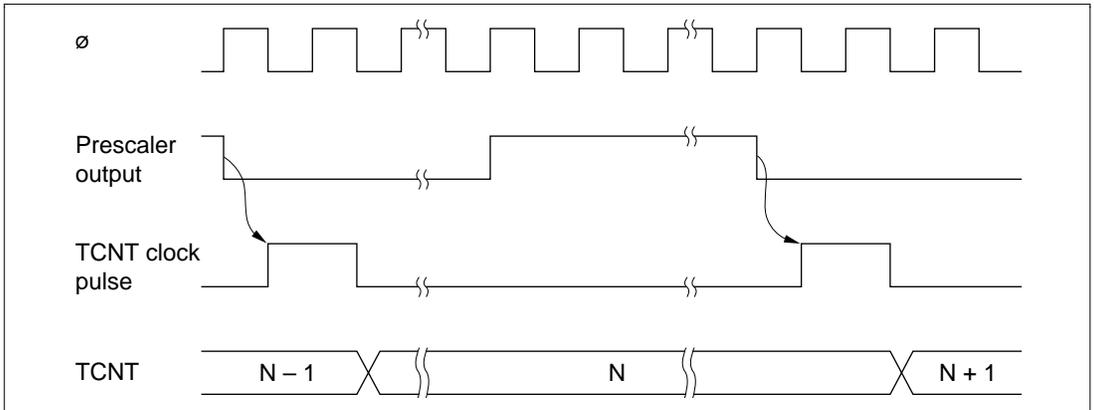
**Figure 10.2 TCNT Increment Timing**
