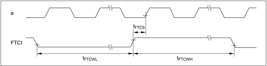
Figure 23.14 External Clock Input Timing for Free-Running Timer
