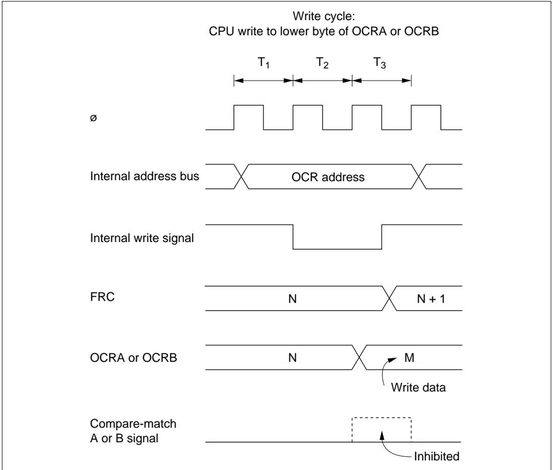
**Figure 8.18 Contention between OCR Write and Compare-Match**
