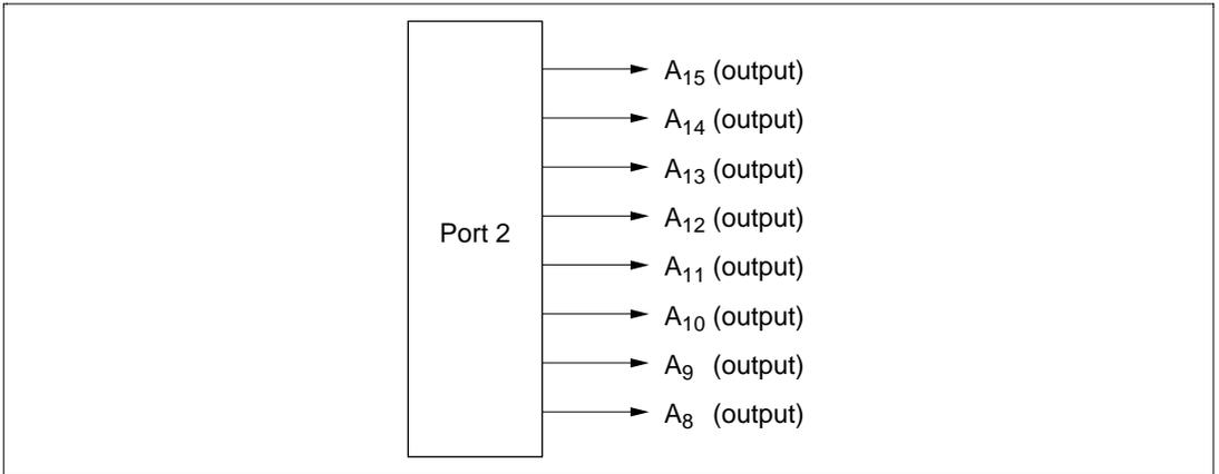
**Figure 7.6 Pin Functions in Mode 1 (Port 2)**
