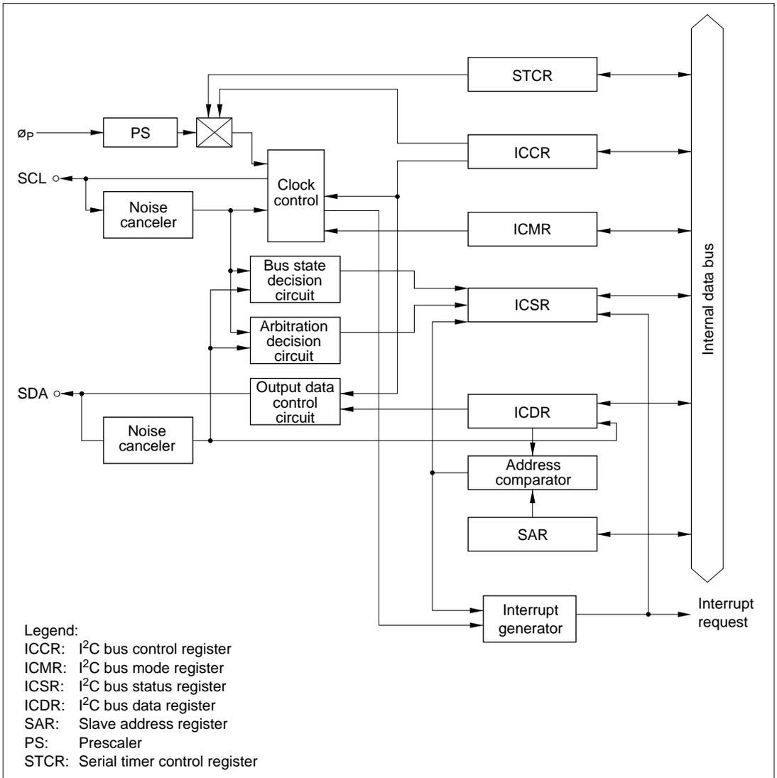
**Figure 13.2 Block Diagram of I<sup>2</sup>C Bus Interface**
