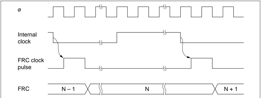
**Figure 8.4 Increment Timing for Internal Clock Source**
