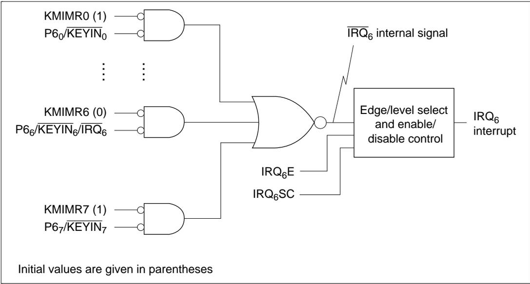
**Figure 4.3 KMIMR and IRQ<sub>6</sub> Interrupt**
