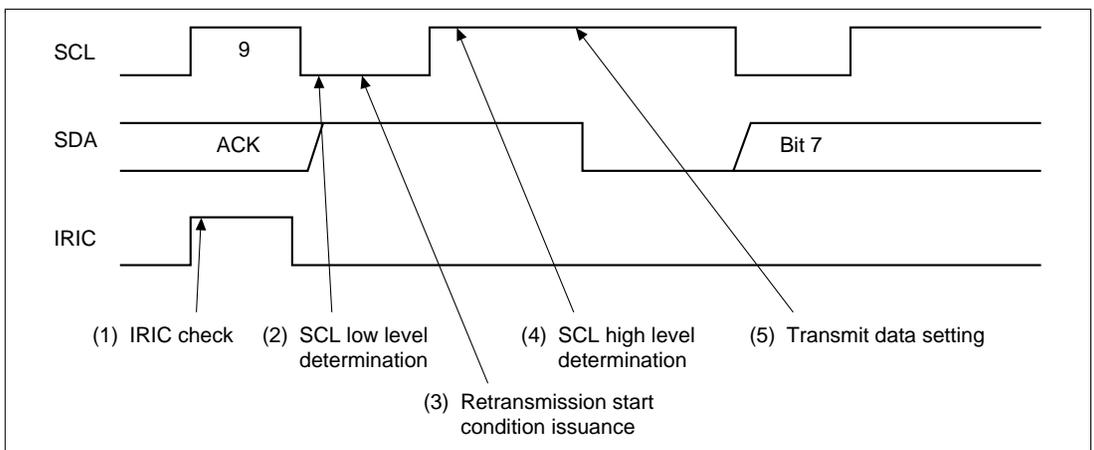
**Figure 13.17 Timing Chart for Retransmission Start Condition Issuance**
