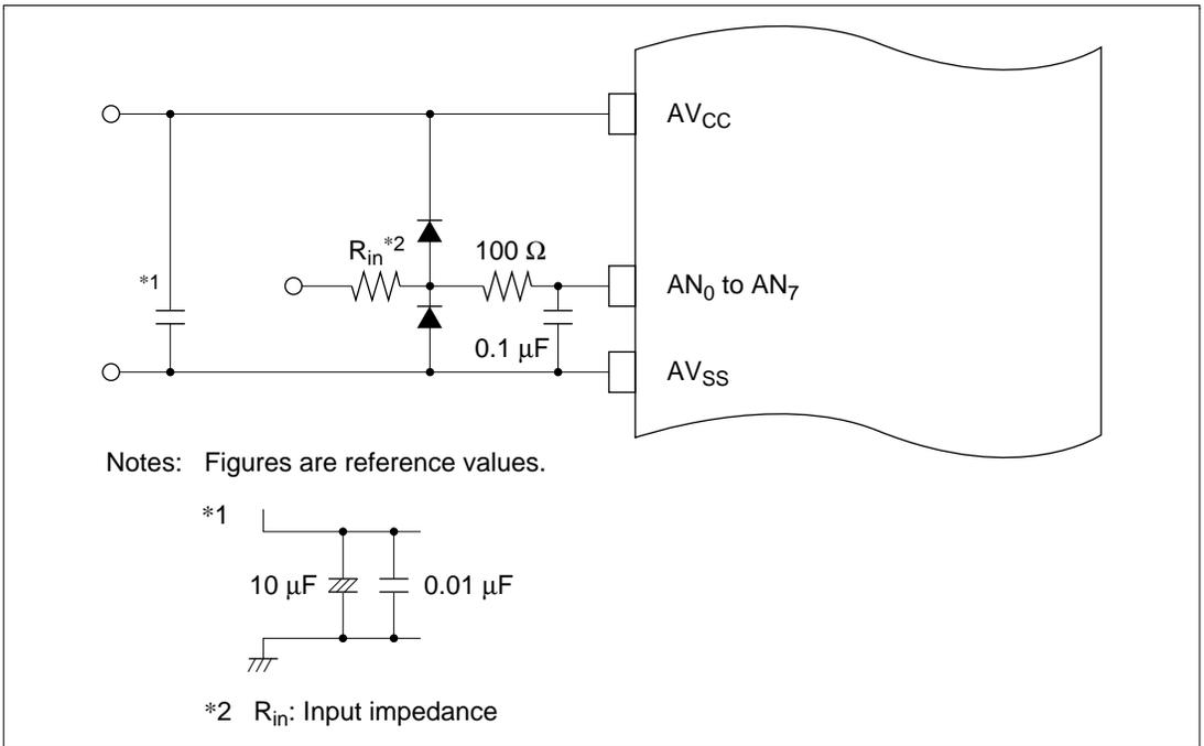
**Figure 15.7 Example of Analog Input Pin Protection Circuit**
