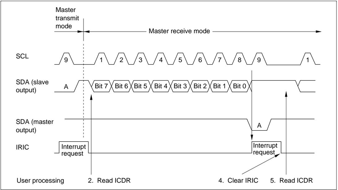
**Figure 13.7 Operation Timing in Master Receive Mode**
