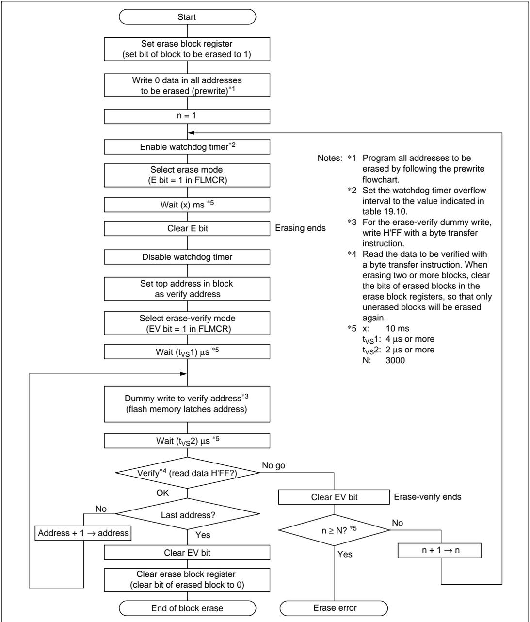
Figure 19.9 Erasing Flowchart
