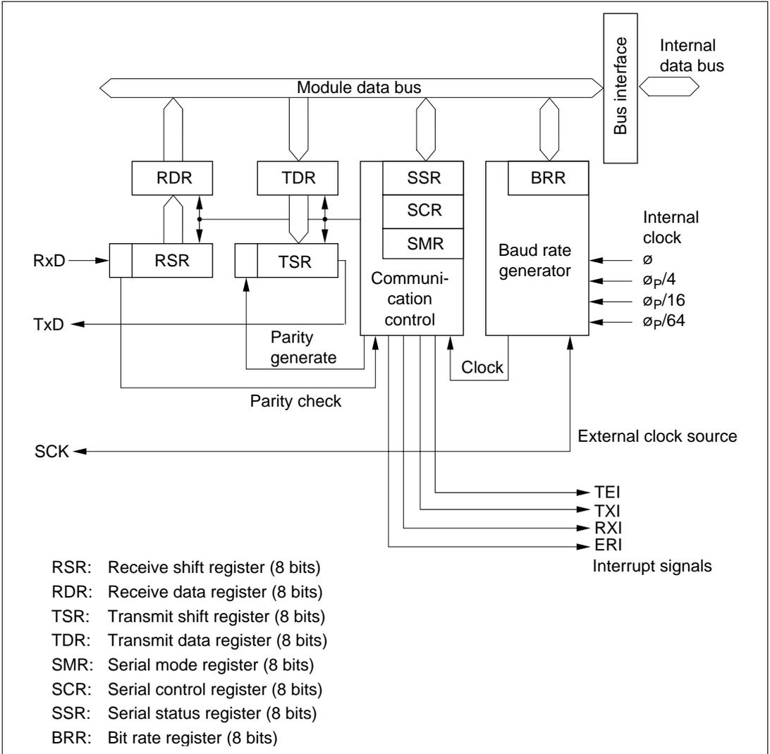
**Figure 12.1 Block Diagram of Serial Communication Interface**
