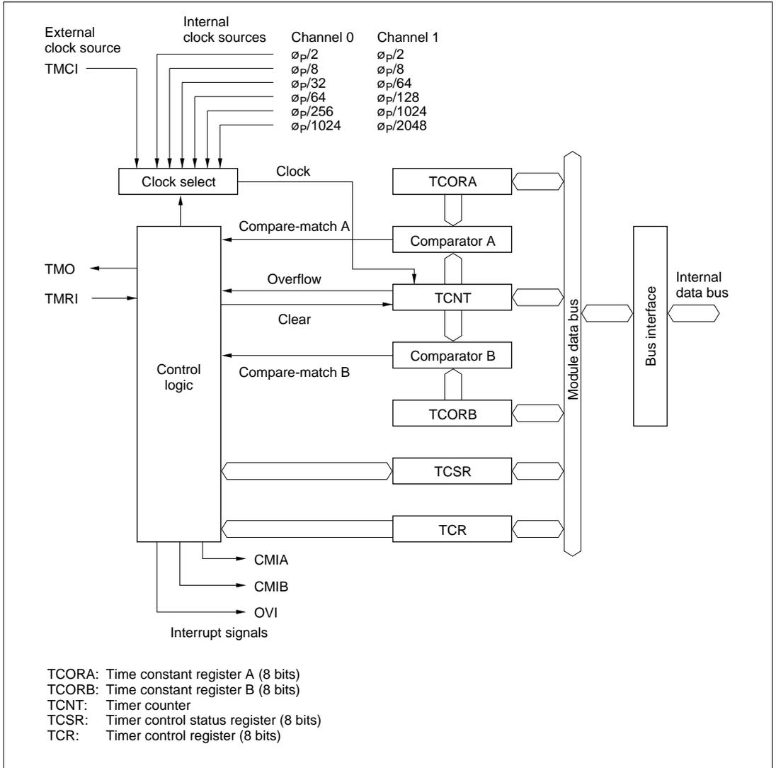
**Figure 9.1 Block Diagram of 8-Bit Timer (1 Channel)**
