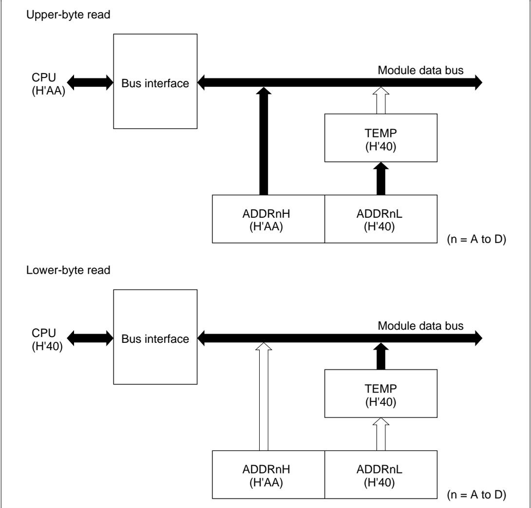
**Figure 15.2 A/D Data Register Access Operation (Reading H'AA40)**
