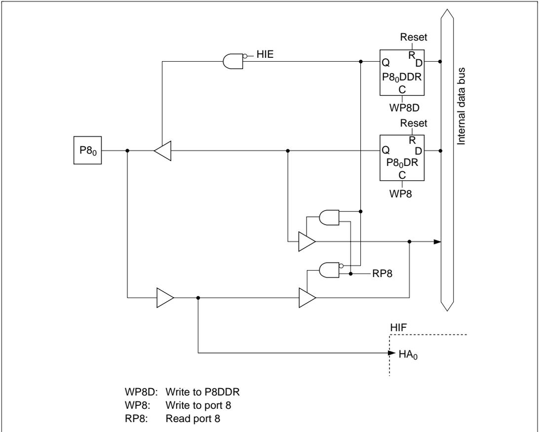
**Figure C.8 (a) Port 8 Block Diagram (Pin P8<sub>0</sub>)**
