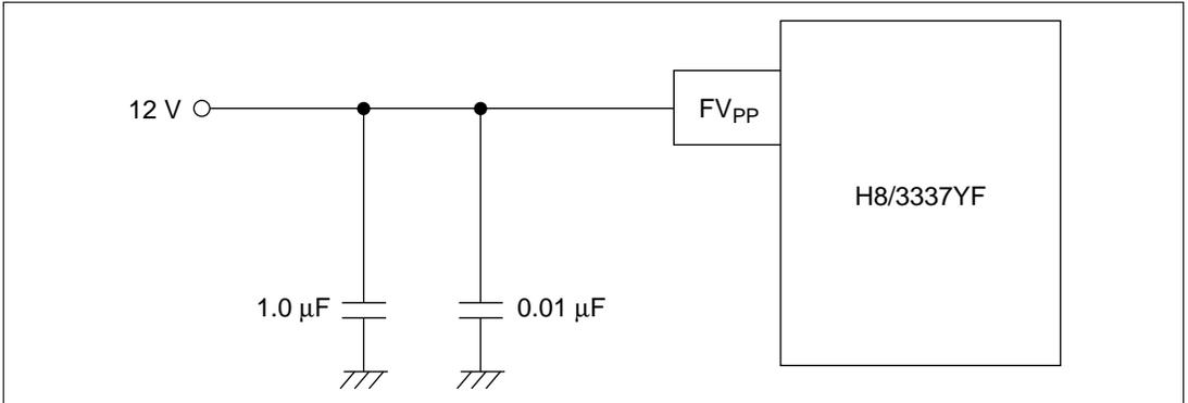
**Figure 20.21  $V_{PP}$  Power Supply Circuit Design (Example)**
