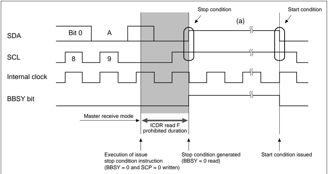
**Figure 13.21 Precautions when Reading Master Receive Data**
