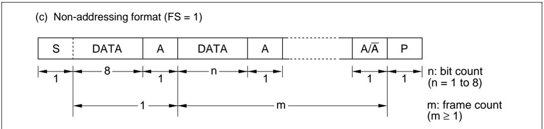
**Figure 13.4 I<sup>2</sup>C Bus Data Format (Non-Acknowledge Format)**
