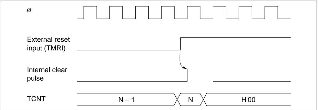
Figure 9.7 Timing of External Reset
