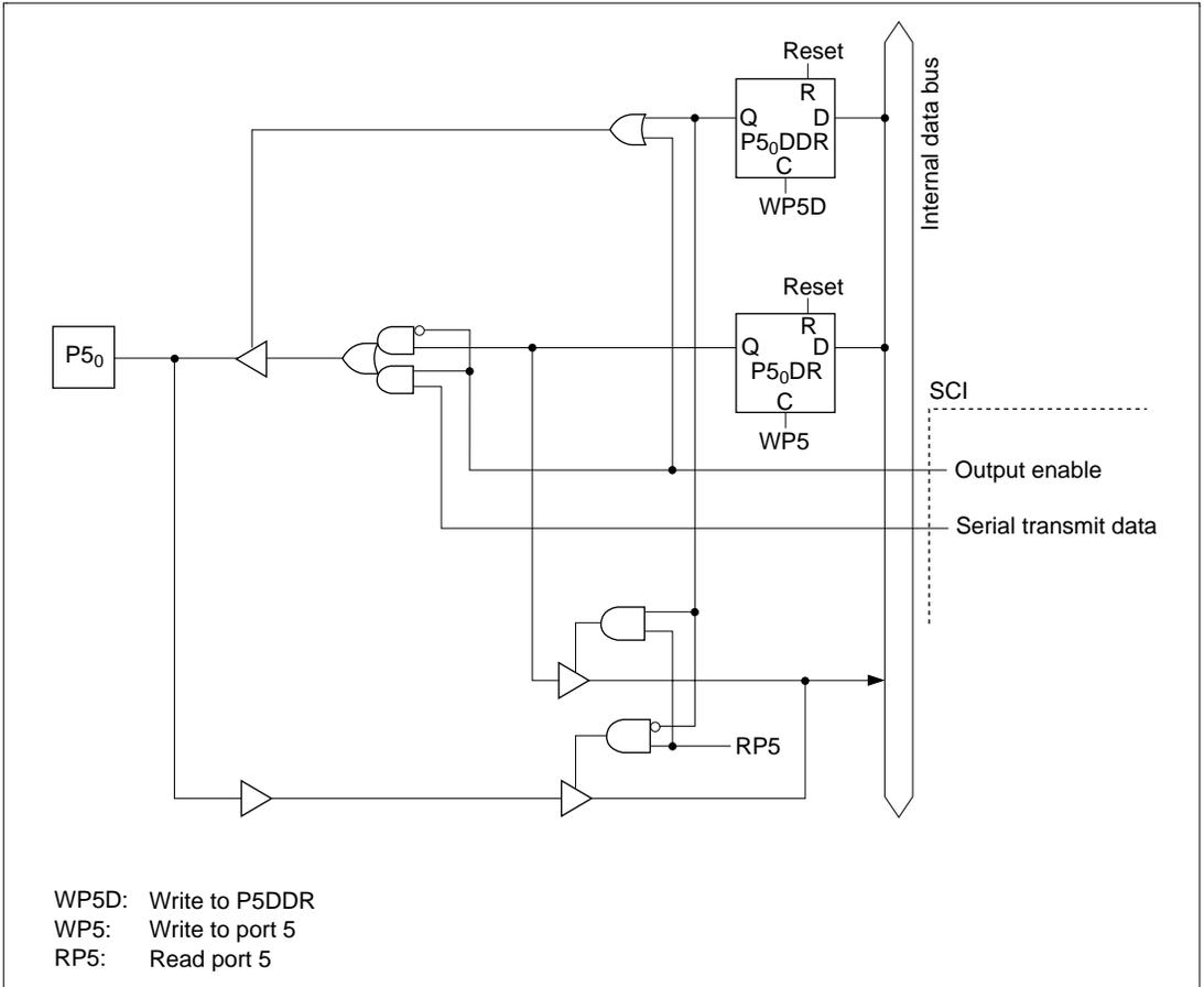
Figure C.5 (a) Port 5 Block Diagram (Pin P5<sub>0</sub>)
