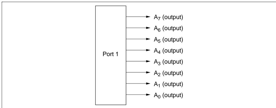
**Figure 7.2 Pin Functions in Mode 1 (Port 1)**
