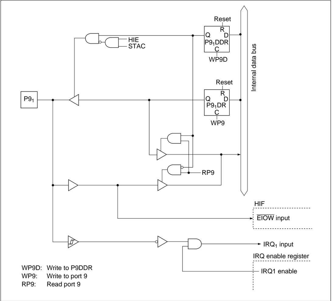
**Figure C.9 (b) Port 9 Block Diagram (Pin P9<sub>1</sub>)**
