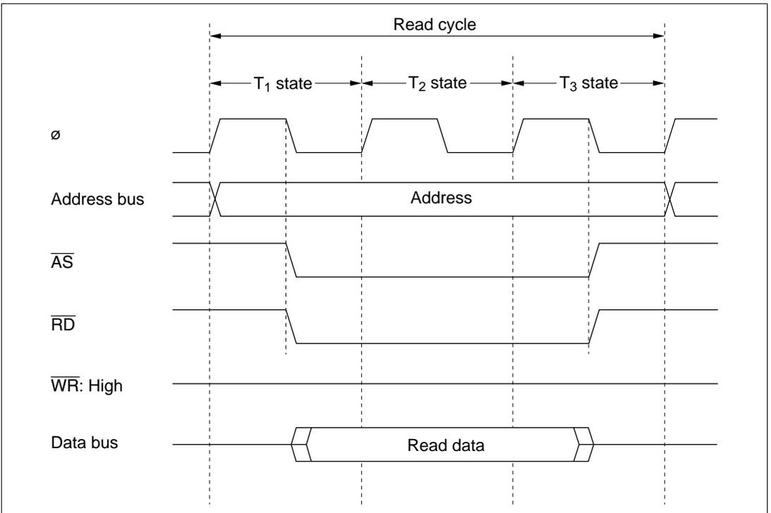
**Figure 2.17 (a) External Device Access Timing (Read)**
