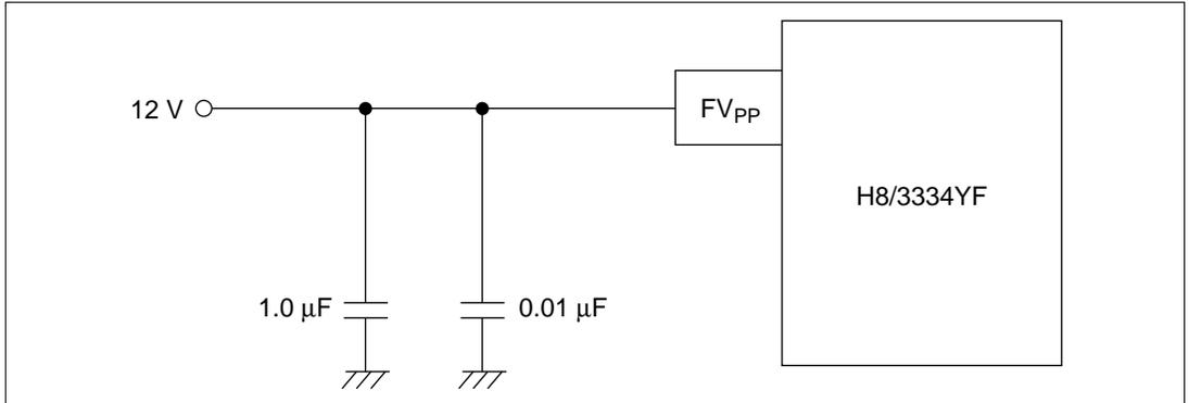
**Figure 19.21  $V_{PP}$  Power Supply Circuit Design (Example)**
