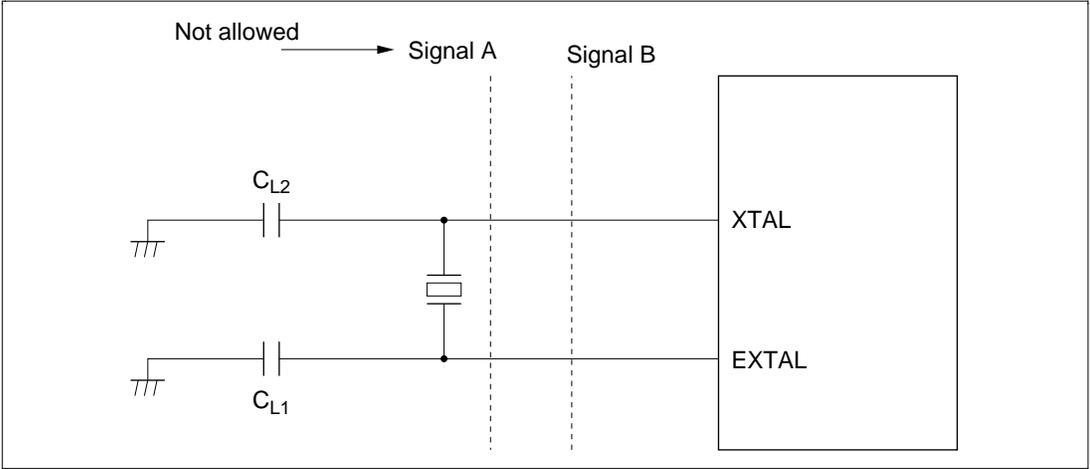
**Figure 6.10 Notes on Board Design around External Crystal**
