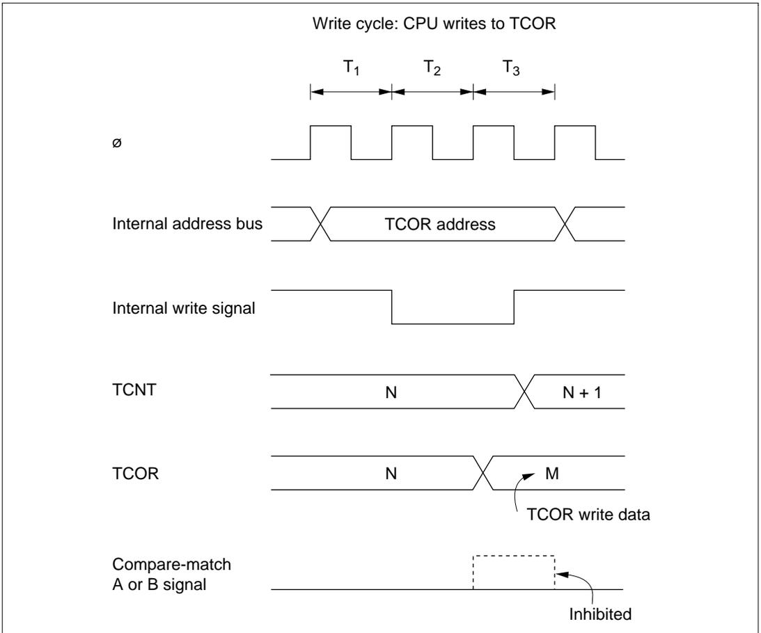
**Figure 9.12** Contention between TCOR Write and Compare-Match
