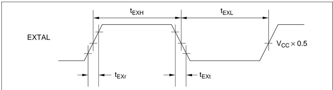
**Figure 6.12 External Clock Input Timing**
