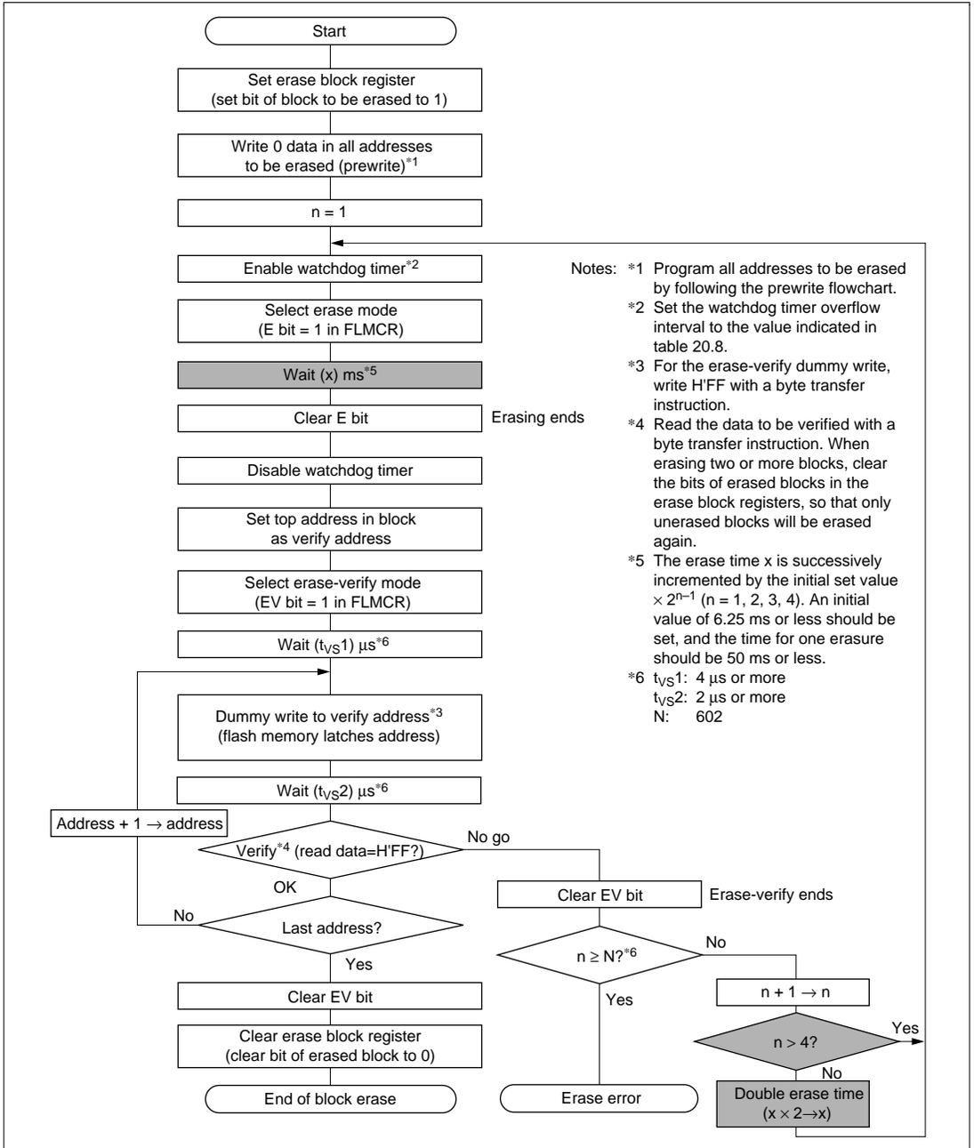
Figure 20.9 Erasing Flowchart
