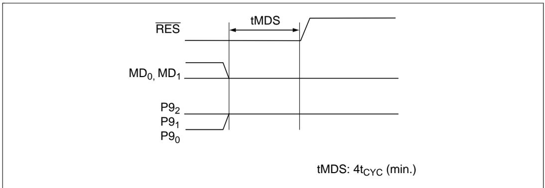
**Figure 21.10 Programming Mode Timing**
