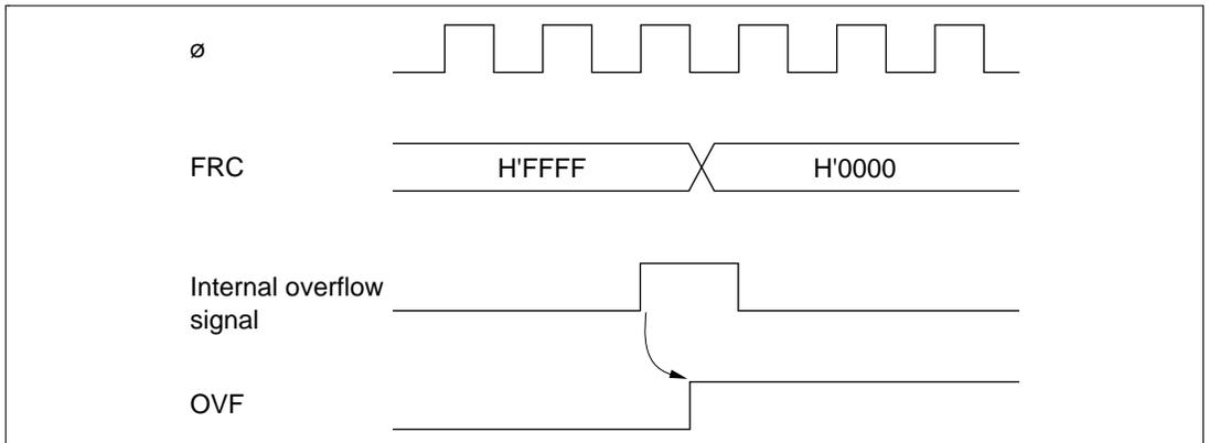
**Figure 8.14 Setting of Timer Overflow Flag (OVF)**
