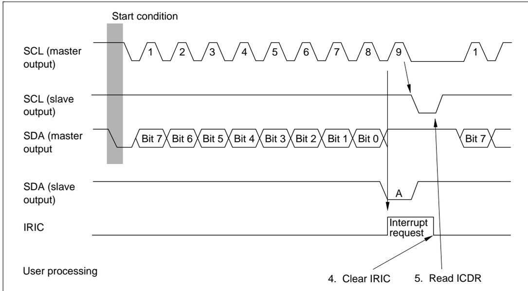
**Figure 13.9 Operation Timing in Slave Receive Mode**
