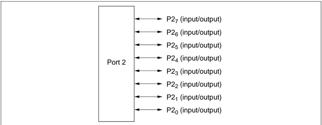
**Figure 7.8 Pin Functions in Mode 3 (Port 2)**
