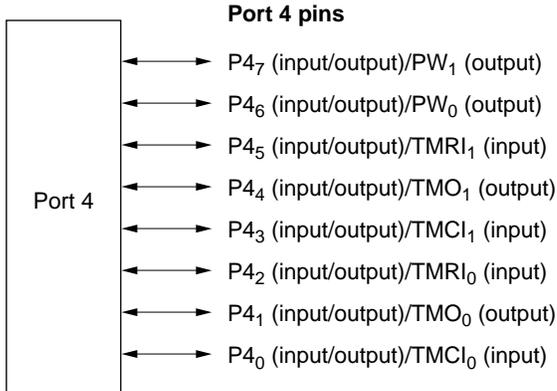
**Pin configuration in mode 3 (single-chip mode)**
