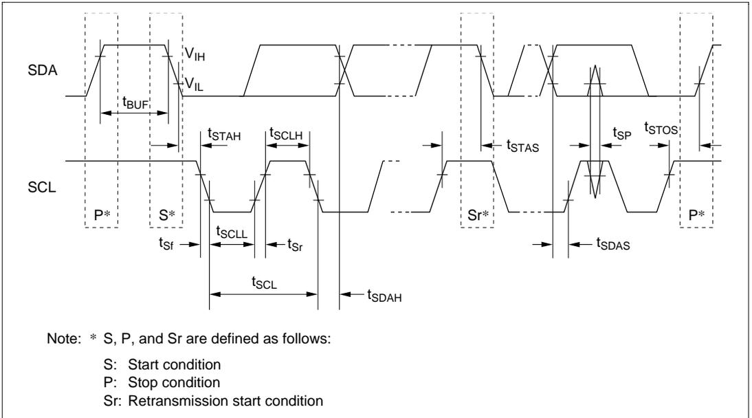
Figure 23.24 I<sup>2</sup>C Interface Input/Output Timing
