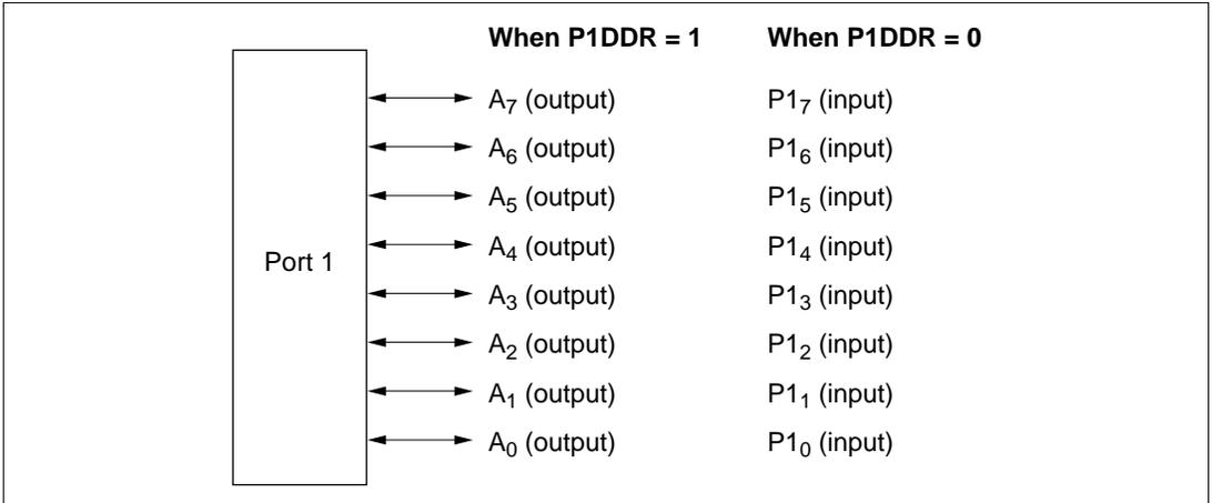
**Figure 7.3 Pin Functions in Mode 2 (Port 1)**
