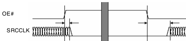
Figure 2. OE# Control Timing
