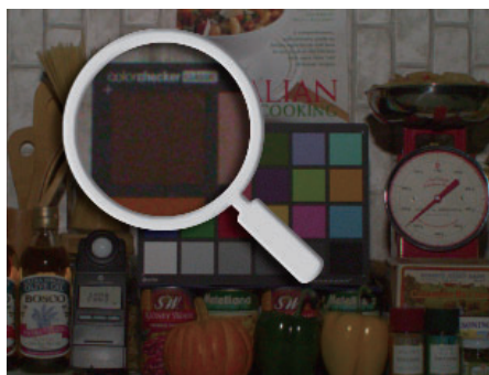
IMX273 (3.75 \mu\text{m} pixels approx. 1.55M effective pixels)
