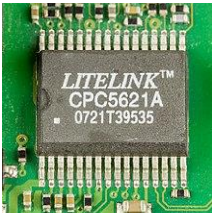
Litelink CPC5621A, a phone line interface IC ( DAA )
