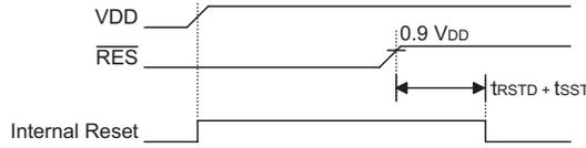
Note:  $t_{RSTD}$  is power-on delay, typical time=50ms
