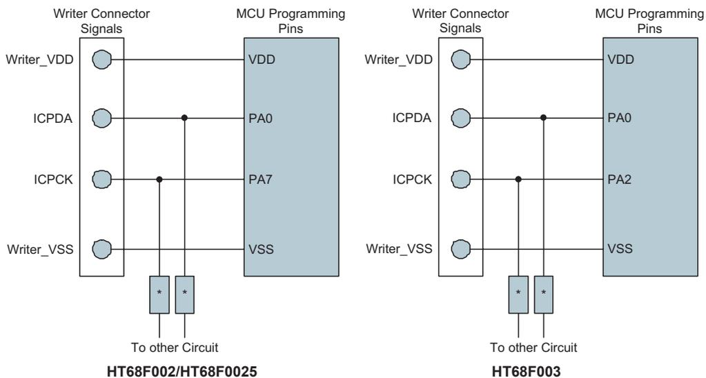
Note: \* may be resistor or capacitor. The resistance of \* must be greater than 1k or the capacitance of \* must be less than 1nF.
