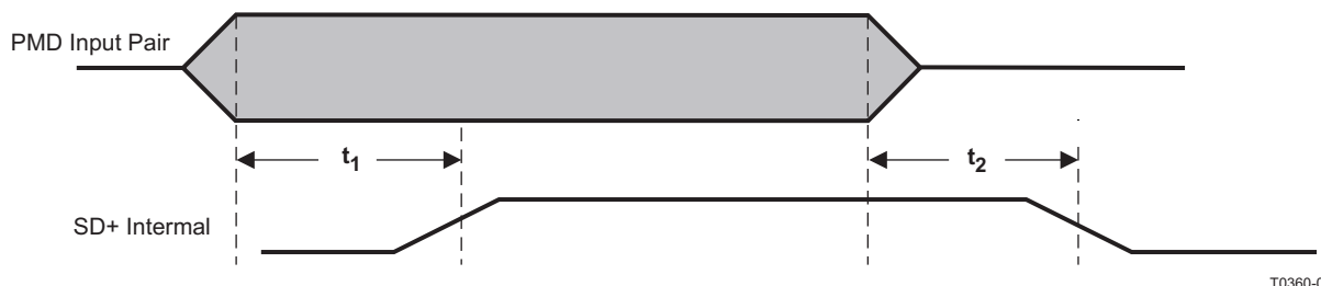
Figure 9-20. 100Base-TX Signal Detect Timing
