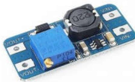
**ICStation MT3608 DC to DC Step Up Converter Module Boost Converter Power Supply Module ICSA004A**
