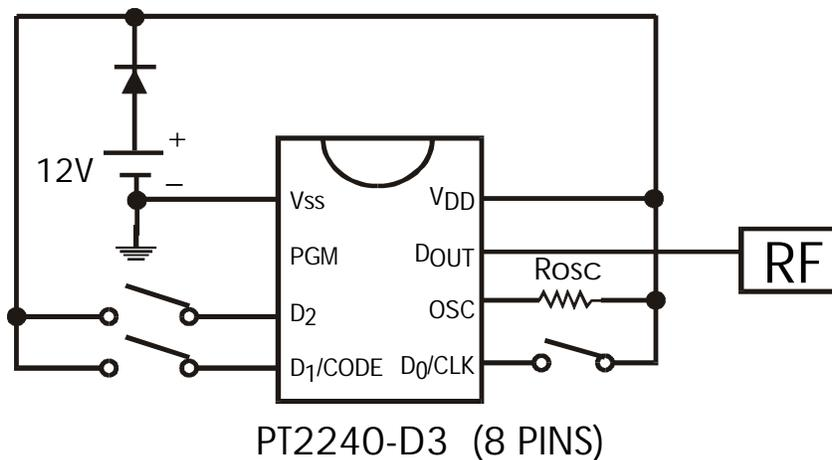
Note: In order that IC protection is assured, please make sure that a diode is connected between the battery and the VDD. If the diode is not connected and the battery polarity was inverted, then the IC will fail.
