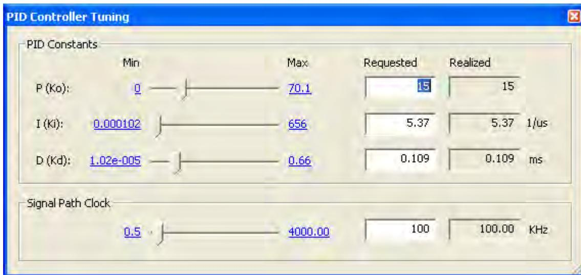
Figure 38 – Fine Tuning Slider Controls - Convenient for Tuning Live Systems
