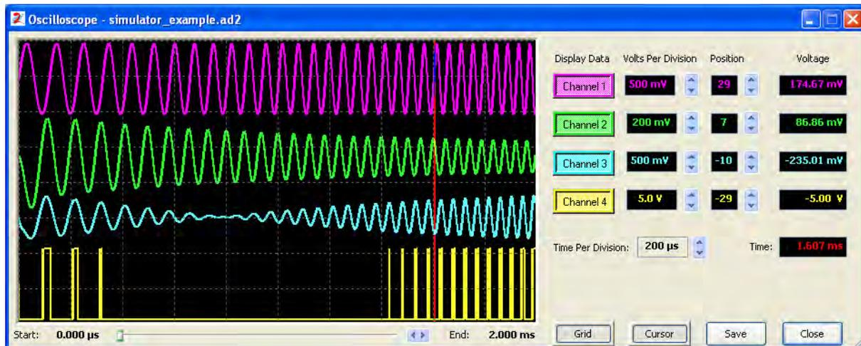
Figure 20 – Oscilloscope Display. High Pass, Swept Input, Band Stop & Comparator signals.
