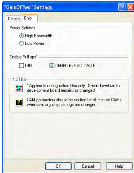
Additional chip level parameters include controls for power consumption, pull-up enables and support for PROM based configuration. As with the parameters in the Clock tab, parameters set in the Chip tab of the dialog box only apply to the chip instance that currently has focus in the design window, the active chip.
