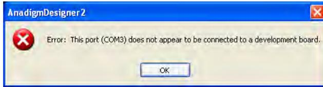
Downloading to the FPAA on an evaluation board is accomplished by selecting the menu item *Configure* → *Write configuration data to serial port*. The download takes approximately 2 seconds. If any communications problems are encountered during the download process, AnadigmDesigner®2 will create a pop-up info window describing the problem.
