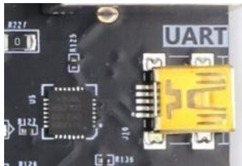
Figure 3-8-2: USB to serial port on the Carrier Board
