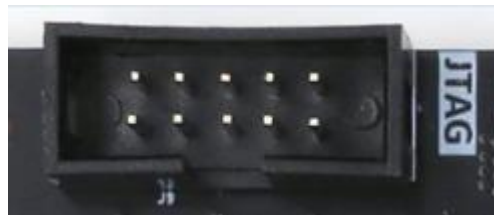
Figure 3-12-2: JTAG Interface on the Carrier Board
