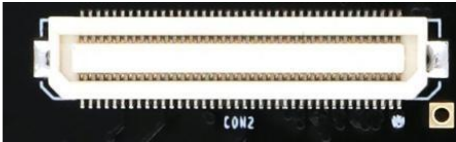
Figure 2-9-2: Board to Board Connectors CON2 on the Core Board
