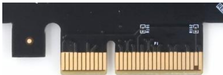
Figure 3-4-2: PCIe x2 on the Carrier Board
