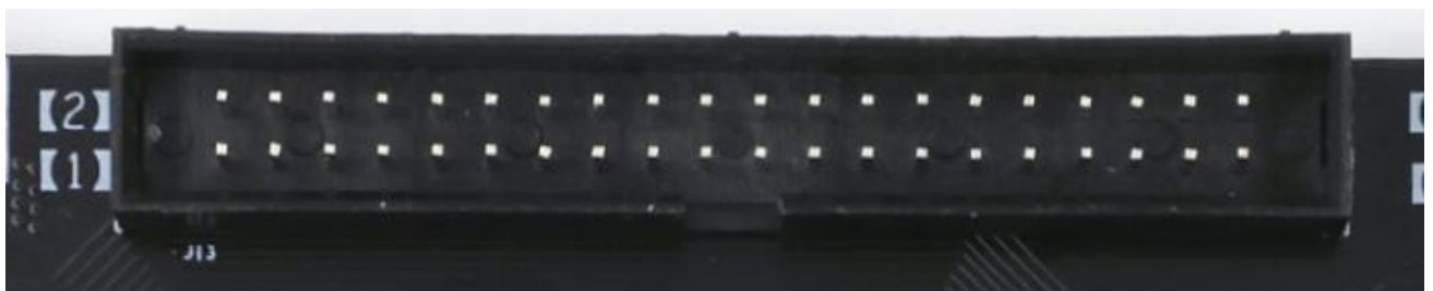
Figure 3-11-4: Expansion header J13 on the carrier board
