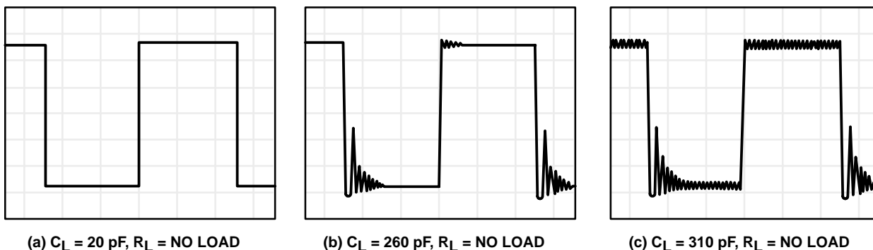
Figure 112. Effect of Capacitive Loads in Low-Bias Mode
