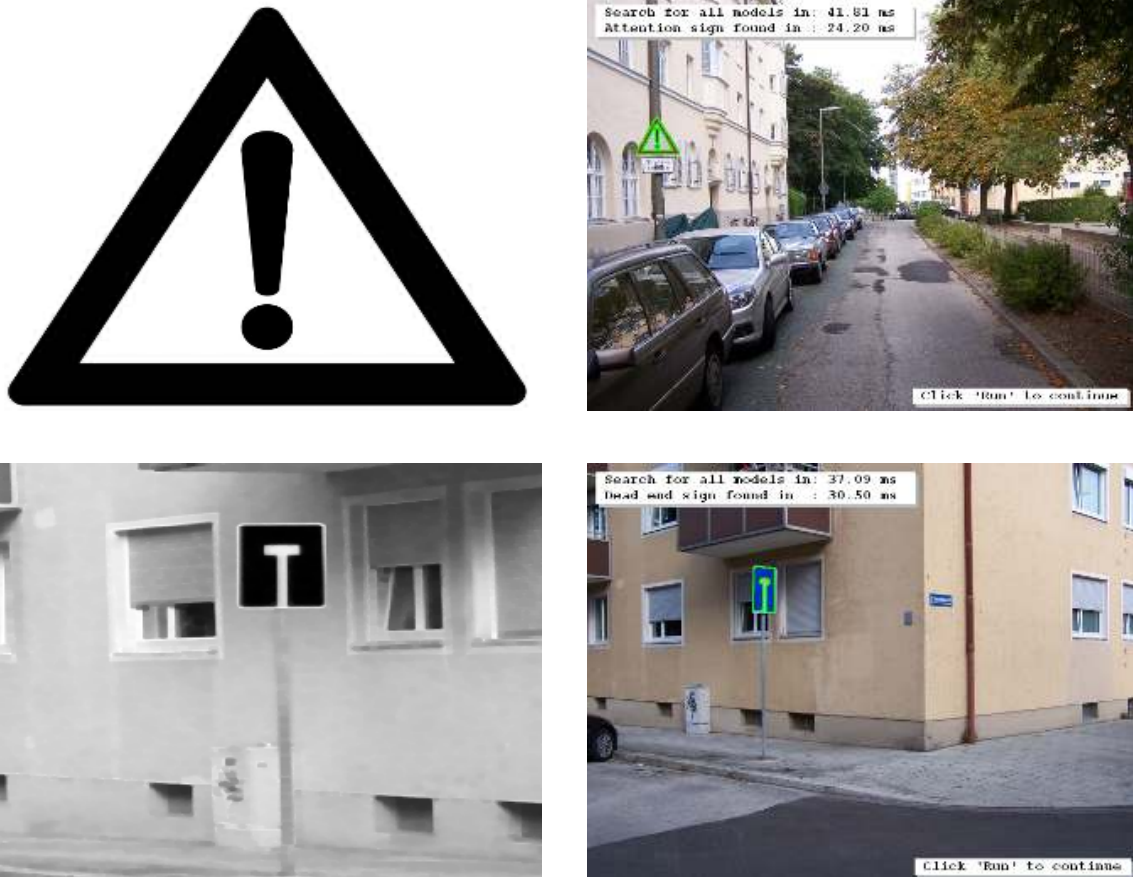
Figure 4.14: Using the models of the attention and the dead end sign, those signs can be tracked in a street.
