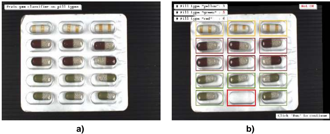
Figure 3.11: (a) The GMM classifier is trained with reference blister image; (b) recognition of a defect, a missing pill.
