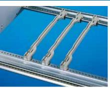
For 160, 220 and 280 mm PCBs up to 2 mm nominal thickness. By installing contact springs, an electrical connection can be made between the PCB and the assembly.
