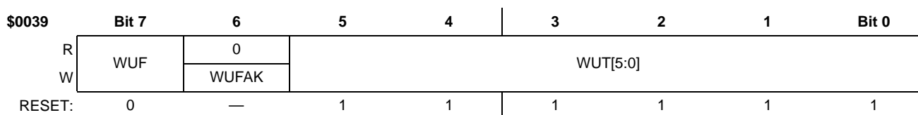
Figure 62. PWU Control/Status Register 0 (PWUCS0)
