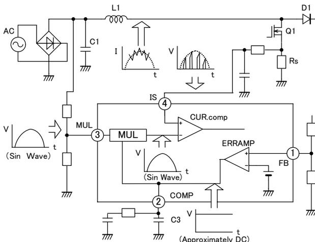
Fig.3 Images of operating waveforms in each part
