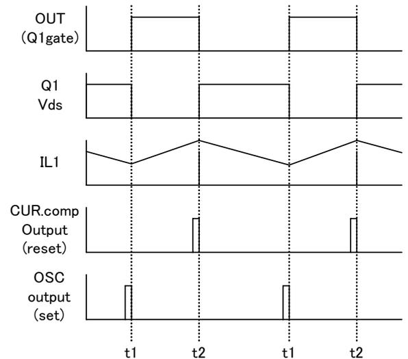
Fig.2 Switching operation; waveforms of each part (Overview)
