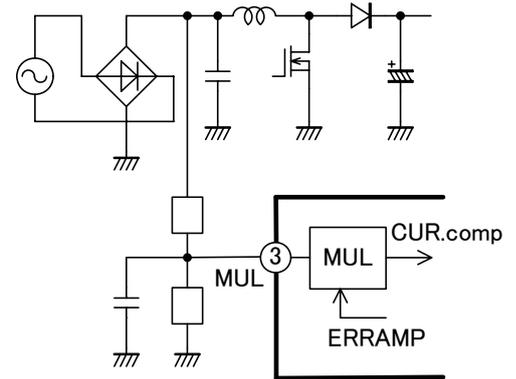
Fig.8 MUL pin circuit
