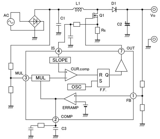
Fig.1 Overview of operating circuit block
