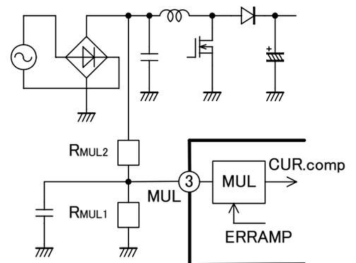
Fig.19 Brownout setting circuit
