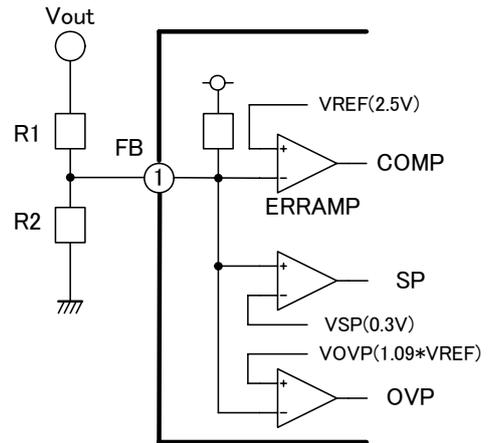
Fig.5 FB pin circuit
