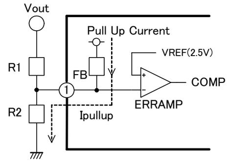
Fig.17 Output voltage setting circuit
