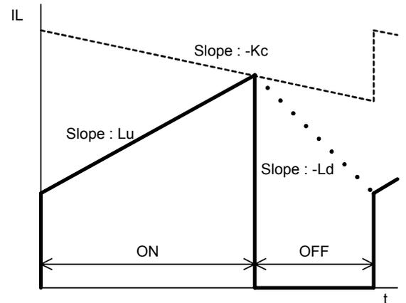
Fig.22 Slope compensation
