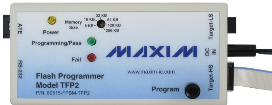
Figure 4-5: Standalone Configuration (shown with Target-HS cable)
