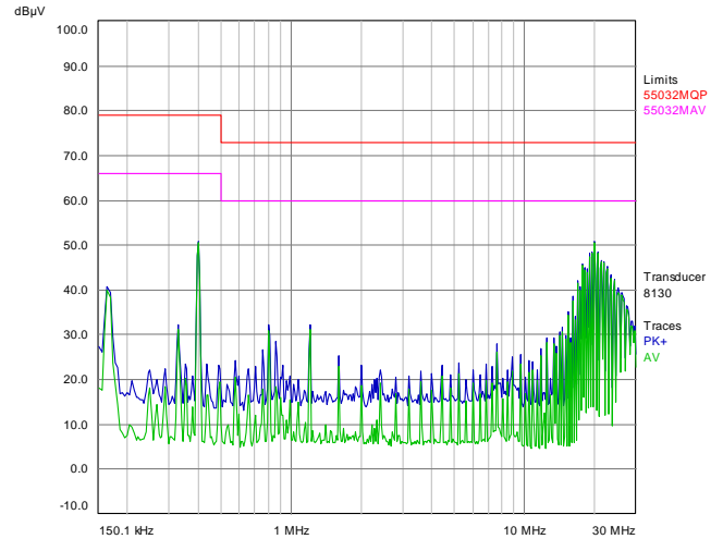
E35SE12013 EN55032 Class A Conducted Emission Test Result
