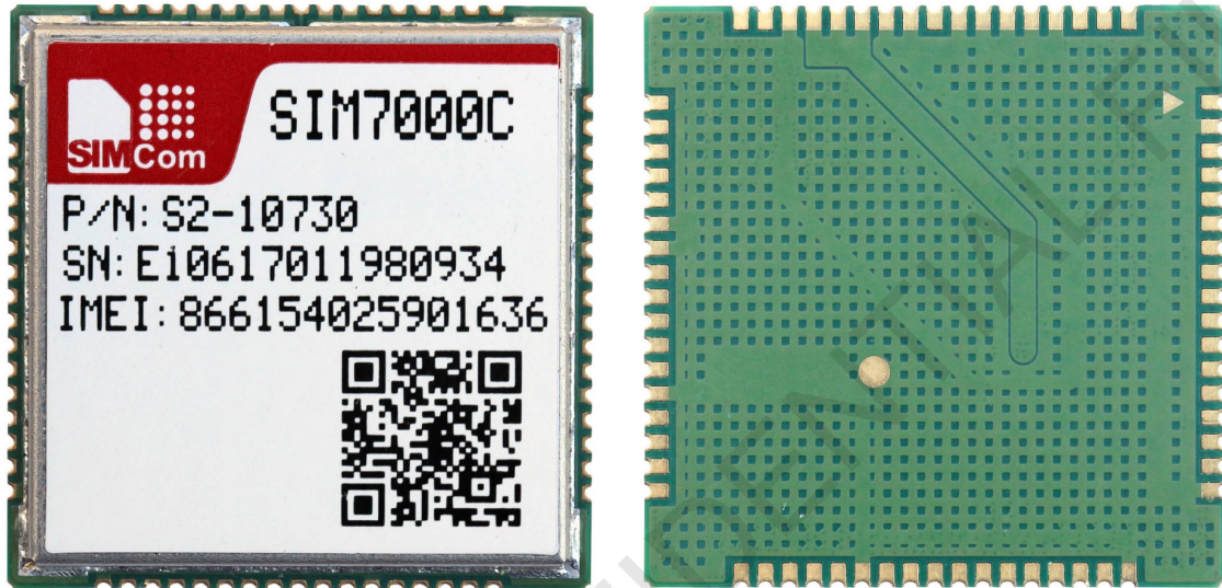
Figure 31: Top and bottom view of SIM7000
