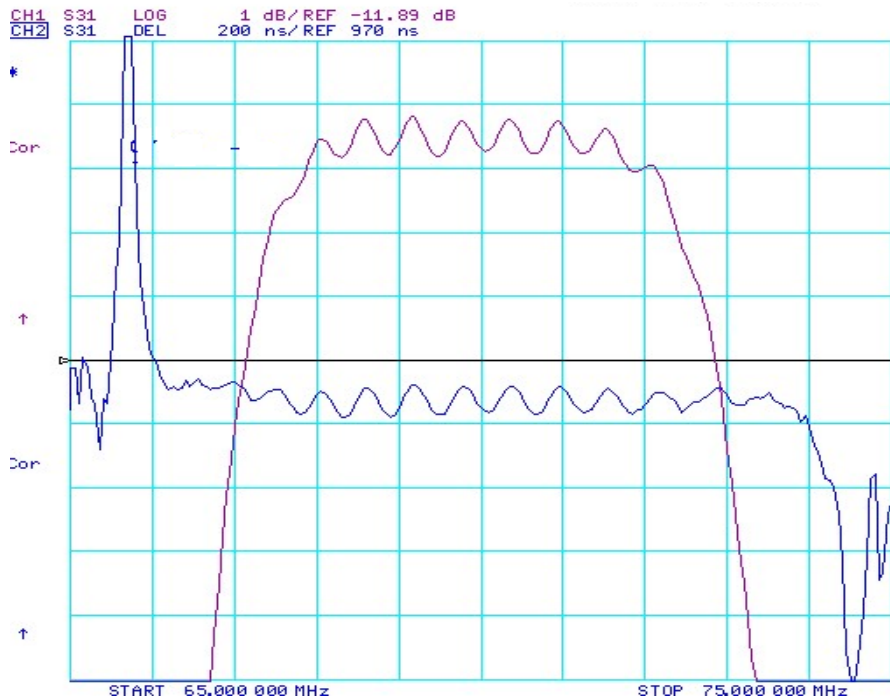
Fig-2 Group Delay and Ripple, Horizontal:1MHz/Div Vertical 1: 1 dB/Div Vertical 2: 200nS/Div
