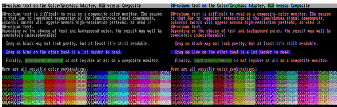
80-column text on RGB (left) vs. composite monitor (right)
