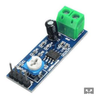
If you want to add audio capabilities to your new project, you could choose the LM386 audio amplifier. It is a high gain audio amplifier based on the LM386 integrated circuit, and it's designed for use in low voltage consumer applications. The gain will increase to any value from 20 to 200 when you put an external resistor and capacitor between pins 1 and 8
