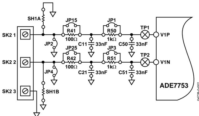
Figure 2. Current Channel on the ADE7753 Evaluation Board
