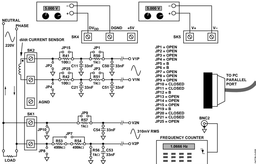
Figure 8. Typical Setup for the ADE7753 Evaluation Board
