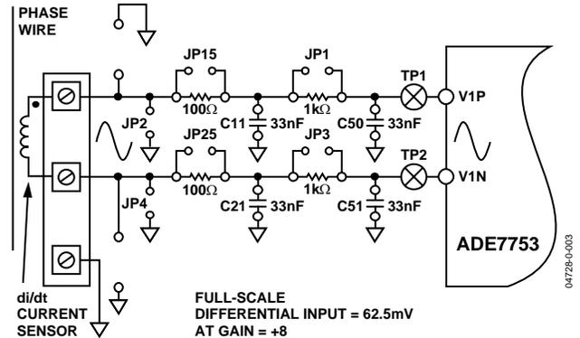
Figure 3. di/dt Sensor Connection to Current Channel
