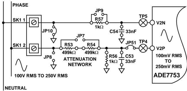
Figure 6. Voltage Channel on the ADE7753 Evaluation Board
