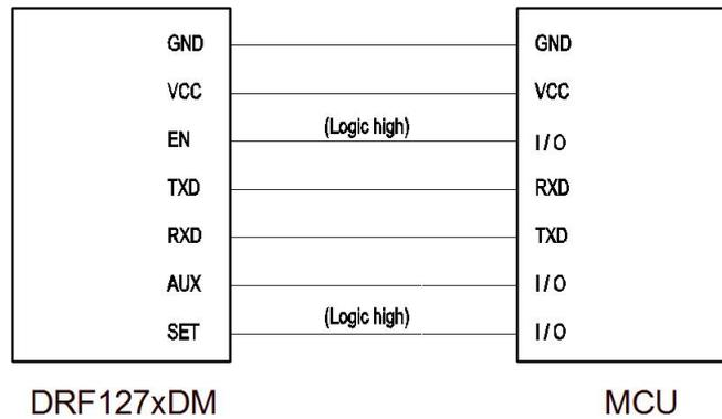
**Figure 3: Node Module in Breath Period Communication**
