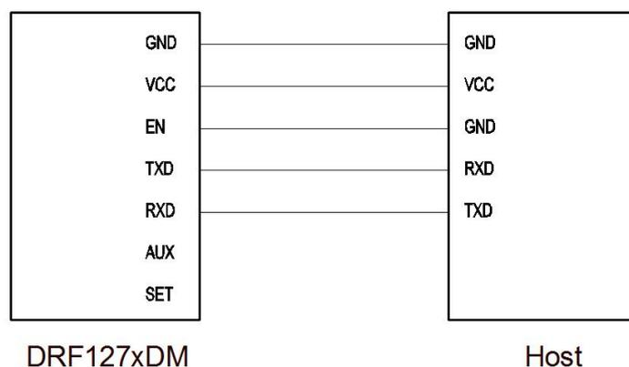
**Figure 6: Pin Connection in Configuring the Module**
