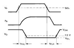
$\label{lem:Figure 26.Propagation delay test waveforms.}$
