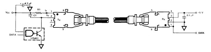
Figure 11. Required 1 MBd interface circuit.
