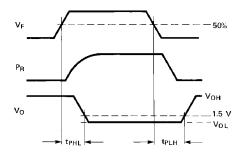
Figure 6. Propagation delay test waveforms.
