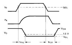
Figure 19. Propagation delay test waveforms.
