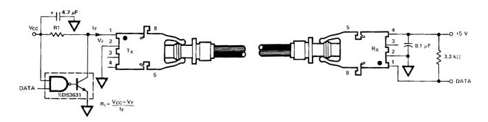
Figure 20. Typical 40 kBd interface circuit.
