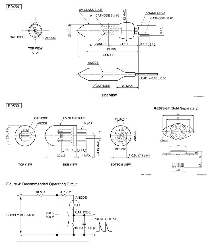
\* This 4.7 k $\Omega$  resistor must be connected within 2.5 cm from the tip of the UVtron anode lead.
