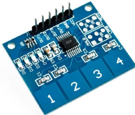
The Capacitive Touch Module 4 Channel TTP224 is a 4 touch key module. It is an innovative way on eliminating the traditional key press button. Within a few millimeters it can detect the finger sense electronically. This allows to simulate the action of button "press". This module is compatible with any [Arduino](#) board.
