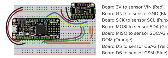
Board 3V to sensor VIN (Red) Board GND to sensor GND (Black) Board SCK to sensor SCL (Purple) Board MOSI to sensor SDA (Green) Board MISO to sensor SDOAG AND sensor DOM (Orange) Board D5 to sensor CSAG (Yellow)
