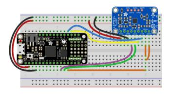
Board 3V to sensor VIN (Red) Board GND to sensor GND (Black) Board SCK to sensor SCL (Purple) Board MOSI to sensor SDA (Green) Board MISO to sensor SDOAG AND sensor SDOM (Orange) Board D5 to sensor CSAG (Yellow) Board D6 to sensor CSM (Blue)
