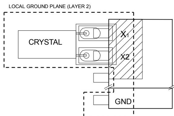
**NOTE:** AVOID ROUTING SIGNAL LINES IN THE CROSSHATCHED AREA (UPPER LEFT QUADRANT) OF THE PACKAGE UNLESS THERE IS A GROUND PLANE BETWEEN THE SIGNAL LINE AND THE DEVICE PACKAGE.
