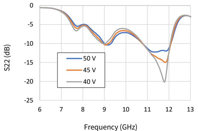
Test conditions unless otherwise noted:  $V_d=45V$ ,  $I_{dq}=1060mA$ , Signal = CW,  $P_{in} = -20dBm$ ,  $T_{base}=25^{\circ}C$
