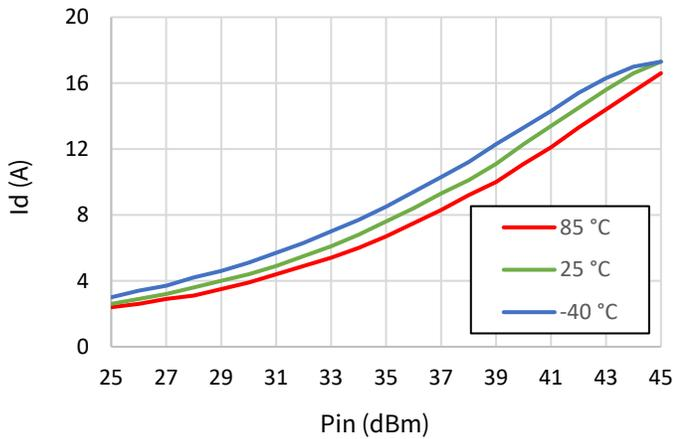
**Figure 26: Ig v. Pin v. Temperature**
