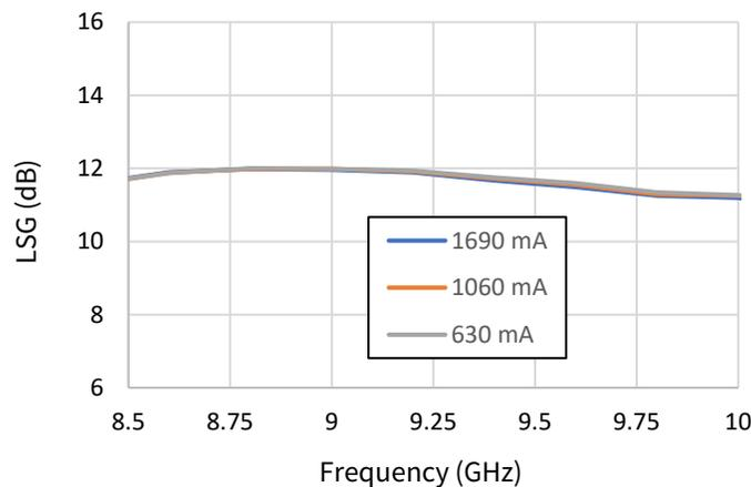
Test conditions unless otherwise noted:  $V_d=45V$ ,  $I_{dq}=1060mA$ ,  $PW=100\mu s$ ,  $DC=10\%$ ,  $P_{in}=43dBm$ ,  $T_{base}=25^\circ C$ , Frequency: 9.5GHz
