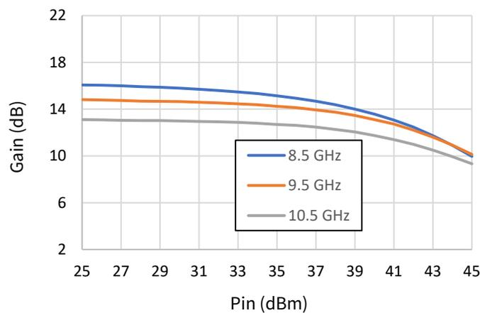
Test conditions unless otherwise noted:  $V_d=45V$ ,  $I_{dq}=1060mA$ ,  $PW=100\mu s$ ,  $DC=10\%$ ,  $P_{in}=43dBm$ ,  $T_{base}=25\text{ }^\circ C$ , Frequency: 9.5GHz
