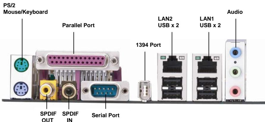
**NOTE:** Peripheral devices can be plugged straight into any of these ports but software may be required to complete the installation.
