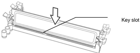
3. Seat the module firmly into the socket by gently pressing down until it sits flush with the socket. The locking levers pop up into place.
