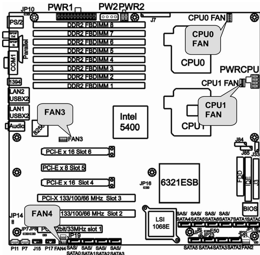
**CPU0FAN/ CPU1FAN/ FAN3/ FAN4: 4-pin FAN Header**
