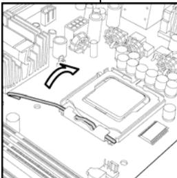
5. Repeat this procedure for the second processor socket.
