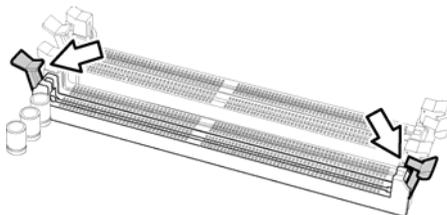
2. Align the memory module with the socket. The memory module is keyed to fit only one way in the socket.
