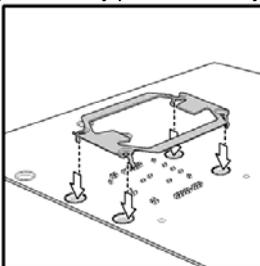
7. Turn the board the right way up again and screw the heat sink into place.
