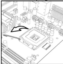
3. Lift the metal cover to expose the socket interior and place the socket in as shown.
