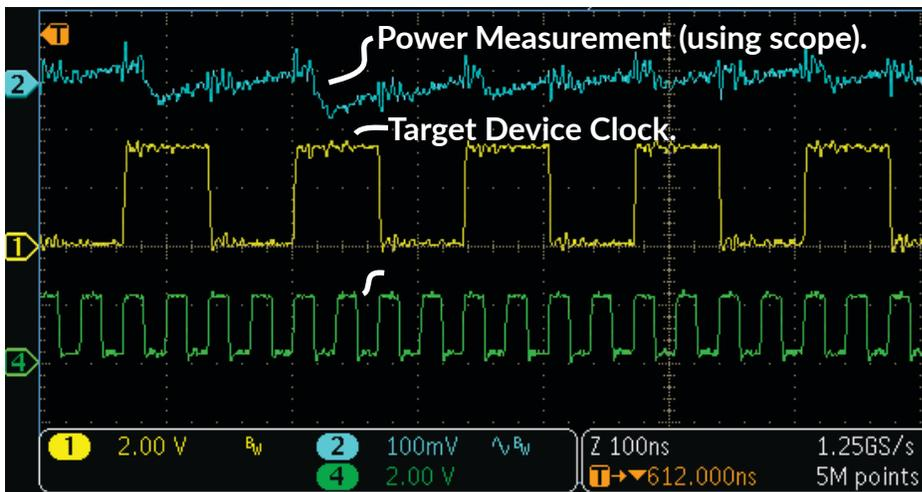
Our ChipWhisperer capture hardware can use a target device clock and apply multiplications and phase shifts to sample at desired point(s) during the clock cycle. This ensures sample points are directly related to the digital clock which generates the signals of interest. The result is many devices can be successfully attacked with 5-100x slower sample clock compared to a regular oscilloscope.
