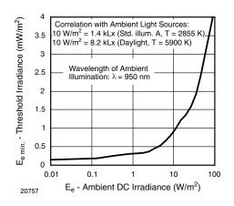
Fig. 6 - Sensitivity in Bright Ambient
