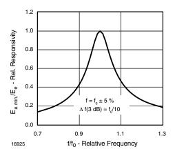
Fig. 5 - Frequency Dependence of Responsivity
