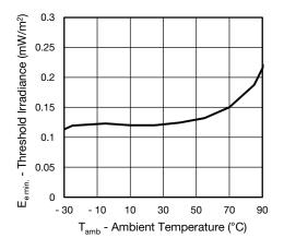
Fig. 9 - Sensitivity vs. Ambient Temperature
