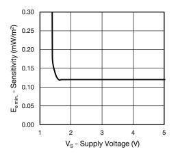
Fig. 13 - Sensitivity vs. Supply Voltage
