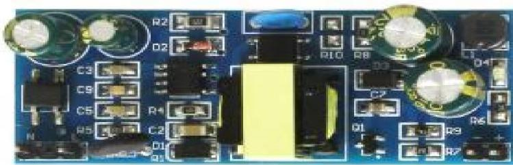
LC THX208 switching power supply module is isolation industrial-grade module .It has function of temperature protection, over current protection and short circuit protection, high and low voltage isolation, AC85 ~ 265 v wide range input voltage, 431 precision voltage stability ,DC5V output.It features small size, stable performance, cost-effective
