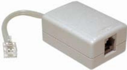
An ADSL filter is required on an ADSL line between each analog device (telephone, fax machine, fax/modem, modem, cordless telephone, alarm dialer etc) and the associated wall outlet. If a filter is not installed, your voice-calls will experience interference whenever ADSL data is being transmitted. Our K2310ASH ADSL Line Filter is ADSL2 and ADSL2+ compatible.
