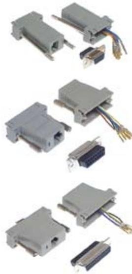
Adapts male or female DB9, DB15 or DB25 computer plugs to 8 position RJ45 or 6 position RJ11 modular socket. Back shell is pre-wired to modular socket ready to insert pins into desired positions of the DB connector.
