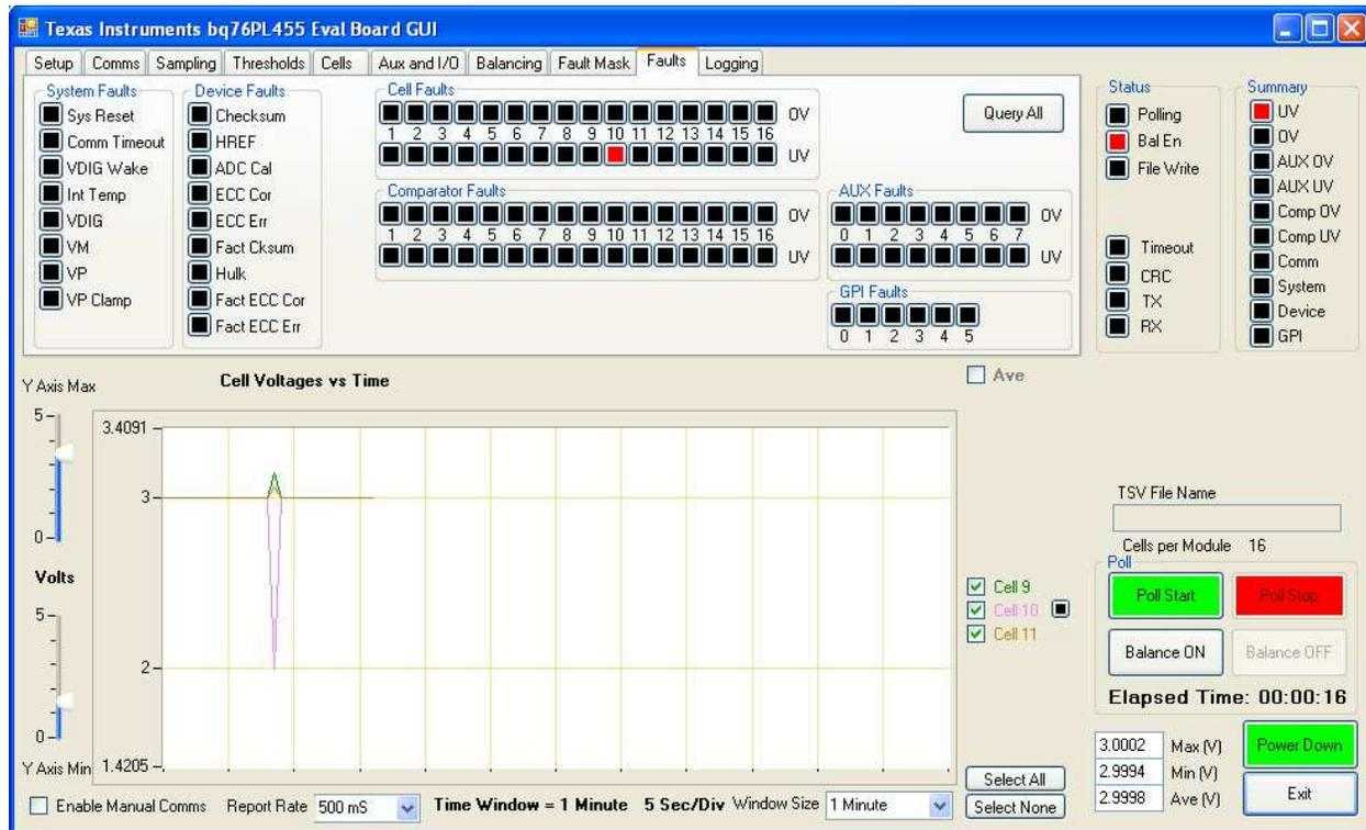
Figure 27. Aborted Balancing Due to UV Fault
