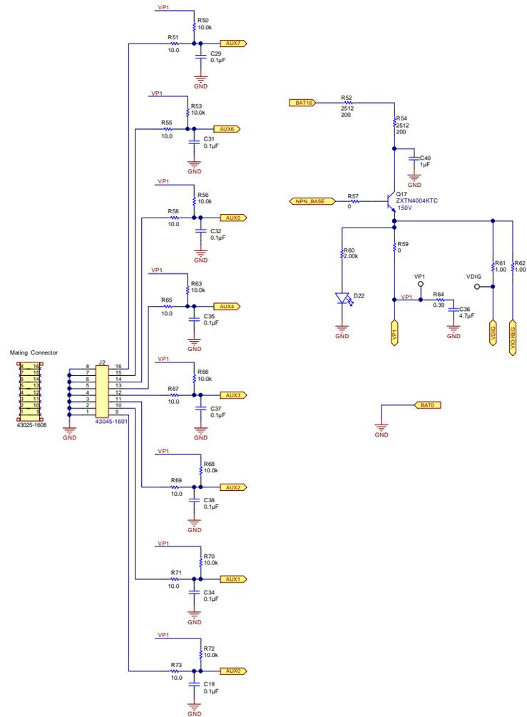
Figure 45. bq76PL455EVM Schematic - Sheet 4
